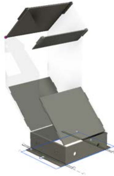
Figure 23. Final Hopper Design
