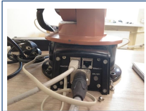
Figure 20. KUKA youBot connections
