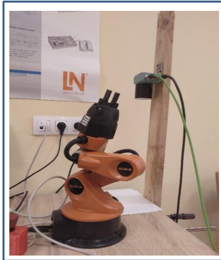
Figure 39. Workspace with robot and camera installed [3.1.2]
