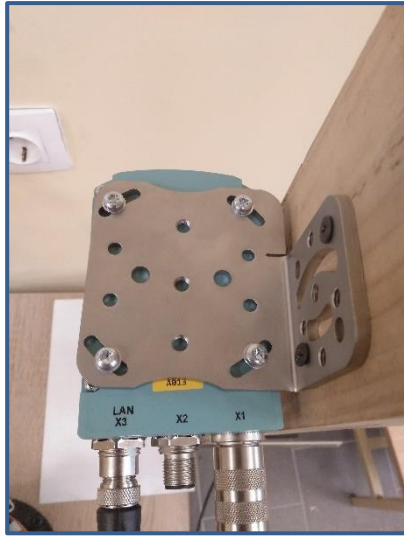
Figure 38. Template and camera screwed to platform[3.1.2]
