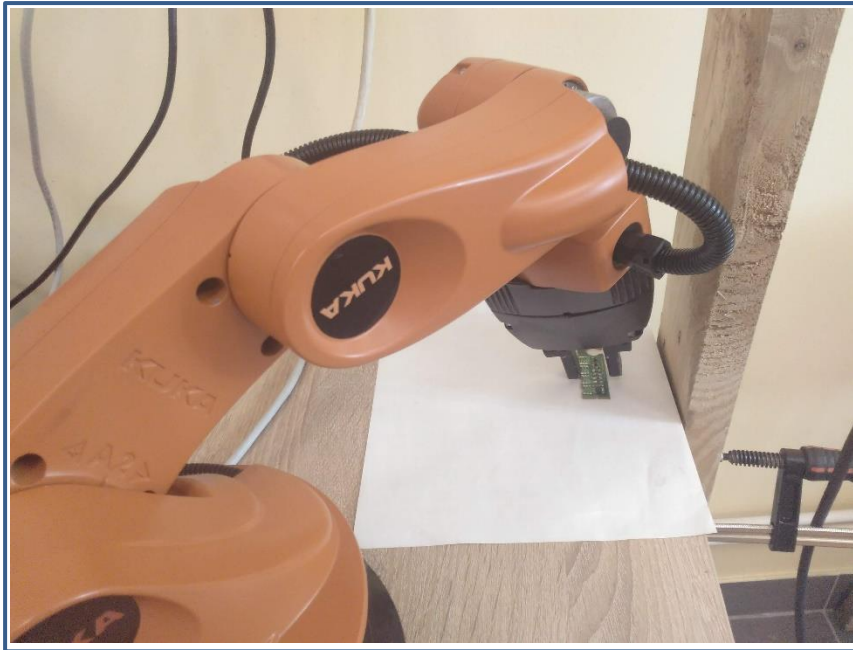
Figure 69. KUKA youBot trying to reach PCB
