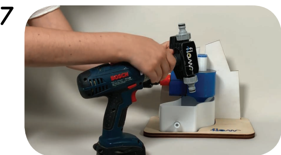
Attach the pump to the drill
