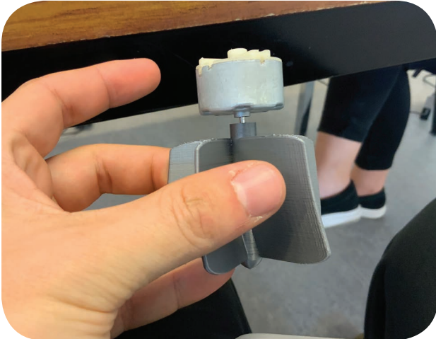
Turbine blade 3D printed
