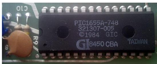
Figura 11. PIC1650 de General Instrument
