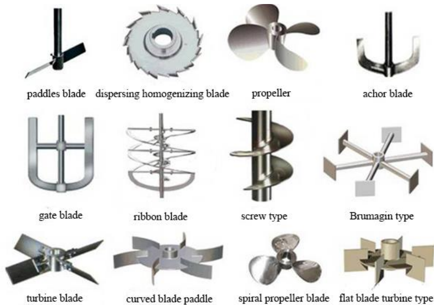
FIGURE 23- SOME EXAMPLES OF DIFFERENT TYPES OF BLADE AGITATORS
