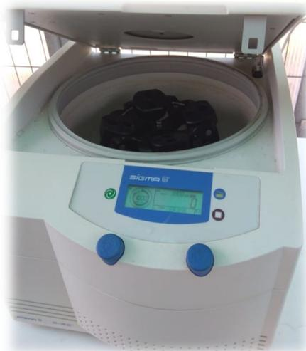
**Figura 6.** Centrífuga SIGMA (2-16P).
