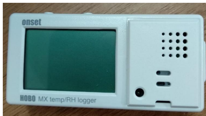
Figure 24: HOBO MX Temp/RH Data Logger (MX1101)
