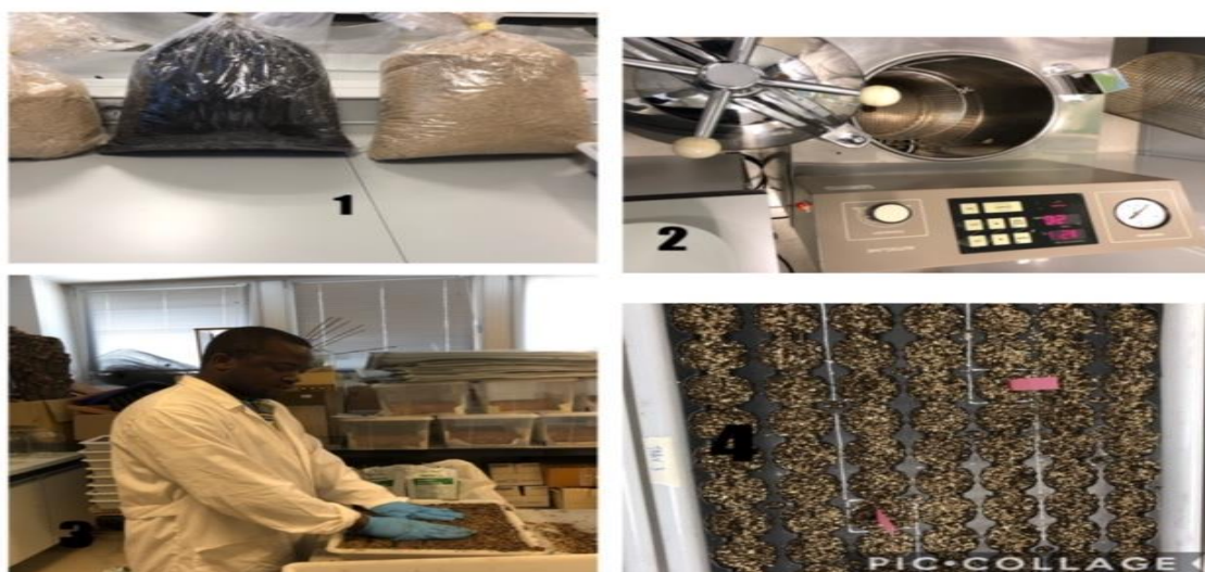
Figure 6: Substrate: (1) +(2) peat moss and vermiculite mixed at 50% and autoclaved; (3) +(4) trays filled with the substrate.
