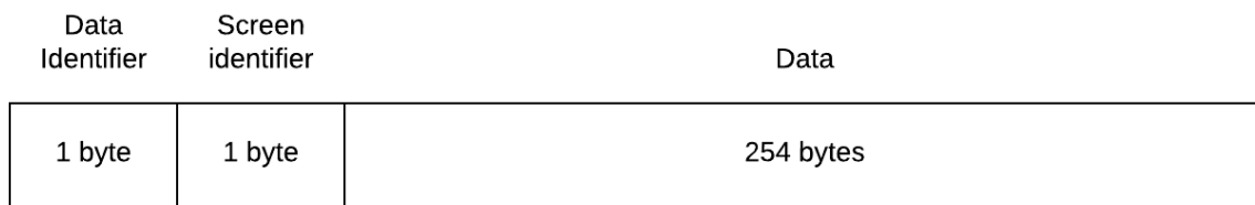
Figure 3.23: UART payload structure
