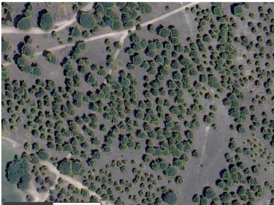
Fig.2 Crown delineation in a mixed stand using the Valbuena et al. (2016) algorithm.
