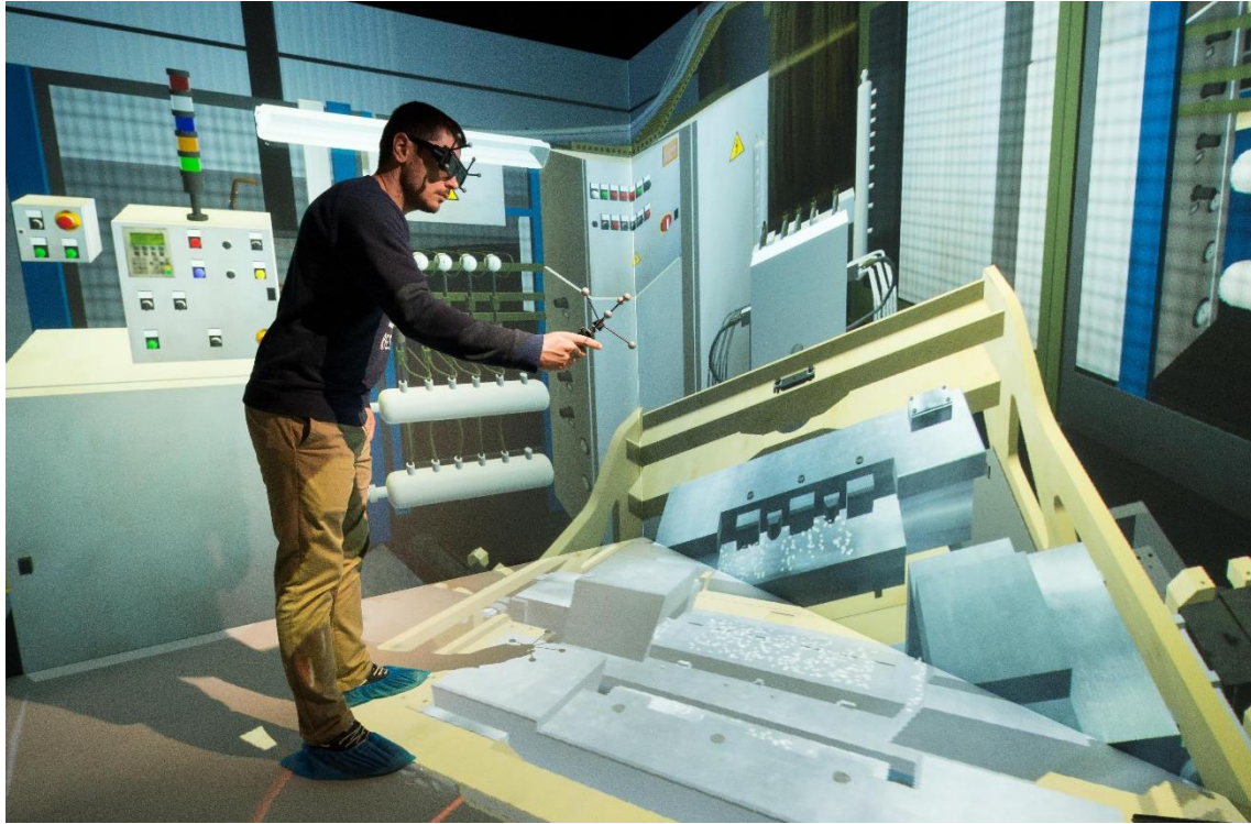
Illustration 21. CAVE System. The user sees in 3D, but we can only see in 3D because we are in a different position (Source: antycipsimulation.com)
