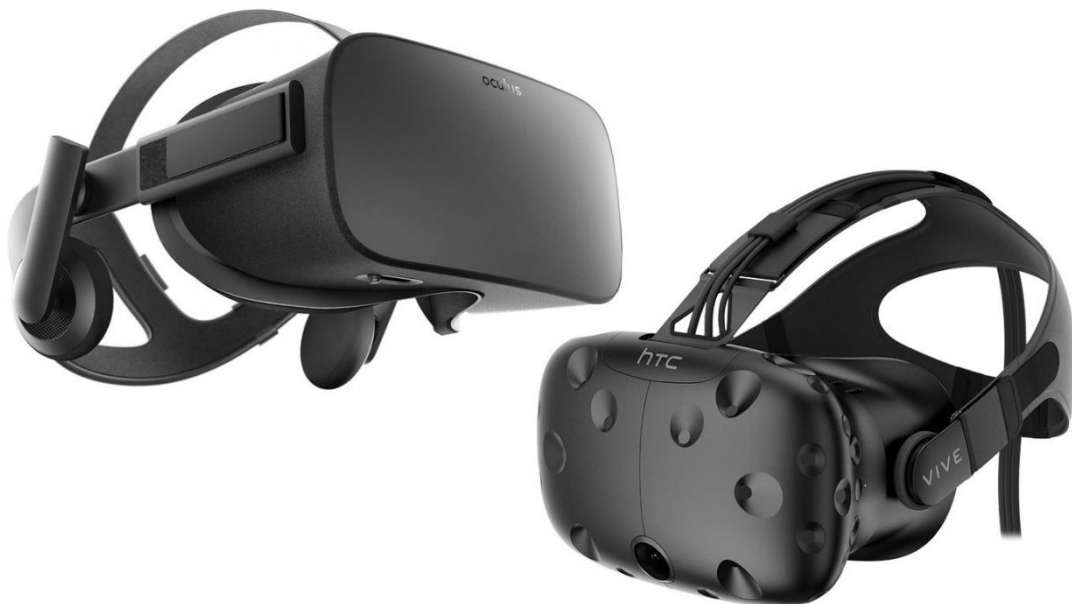
Illustration 22. HMD (Oculus Rift on the left side and HTC Vive on the right side) (Source: gamestar.de)
