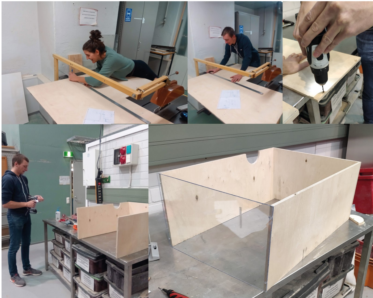
Figure 63 Fish tank support frame building process.
