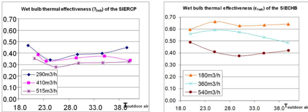
Figure 7. Wet bulb thermal effectiveness variation with outdoor air-dry bulb temperature for the SIERCP and the SIECHB
