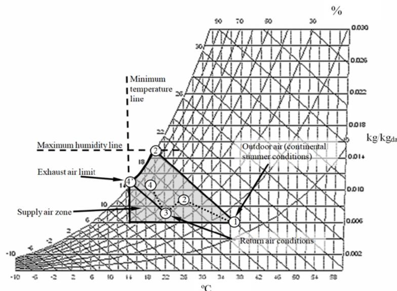
Figure 4. Area of possible evolution of return and outdoor air streams in continental climates (summer conditions), and evolution followed in a generic test.
