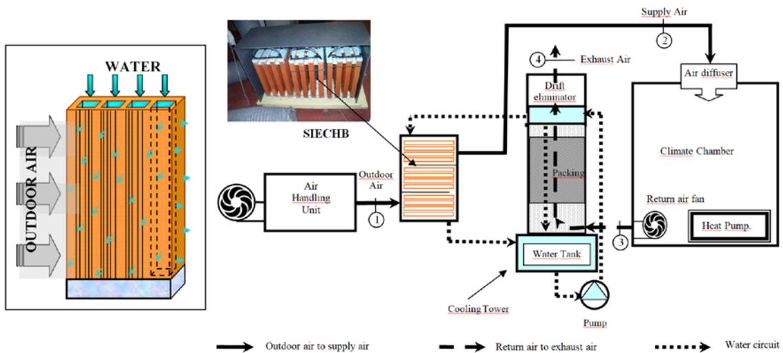
Figure 2. View of the SIECHB, operation, setting and detail of a hollow brick.
