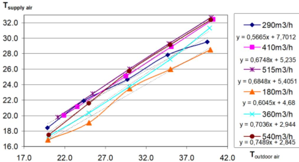
Fig. 5. Supply air dry bulb temperature variation with outdoor air-dry bulb temperature.
