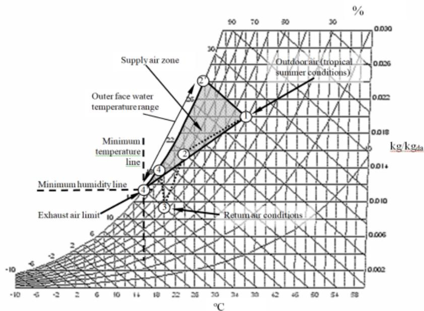
Figure 3. Area of possible evolution of return and outdoor air streams in tropical climates (summer conditions), and evolution followed in a generic test.
