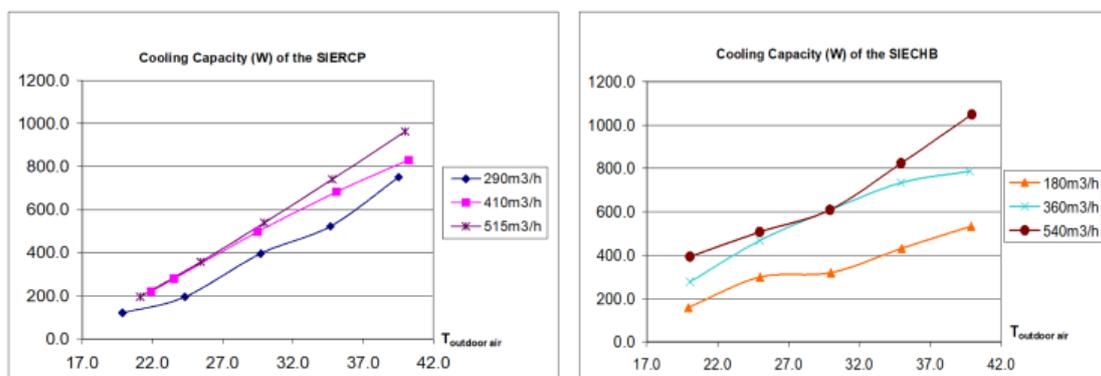
**Figure 6. Cooling capacity variation with outdoor air-dry bulb temperature for the SIERCP and the SIECHB**
