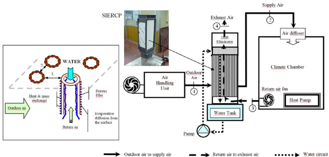
Figure 1. View of the SIERCP, operation and setting.
