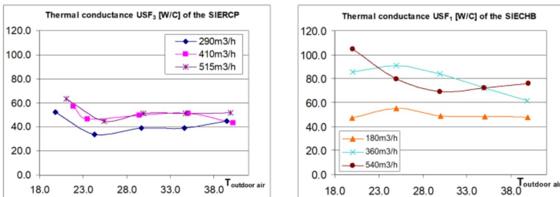
Figure 8. Thermal conductance variation with outdoor air-dry bulb temperature for the SIERCP and the SIECHB
