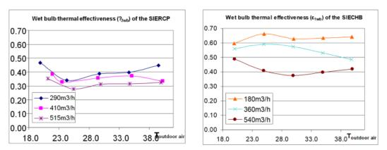
Figure 7. Wet bulb thermal effectiveness variation with outdoor air-dry bulb temperature for the SIERCP and the SIECHB
