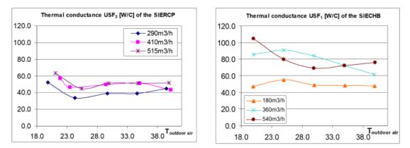
Figure 8. Thermal conductance variation with outdoor air-dry bulb temperature for the SIERCP and the SIECHB
