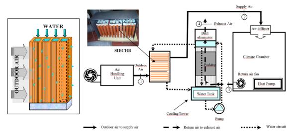
Figure 2. View of the SIECHB, operation, setting and detail of a hollow brick.
