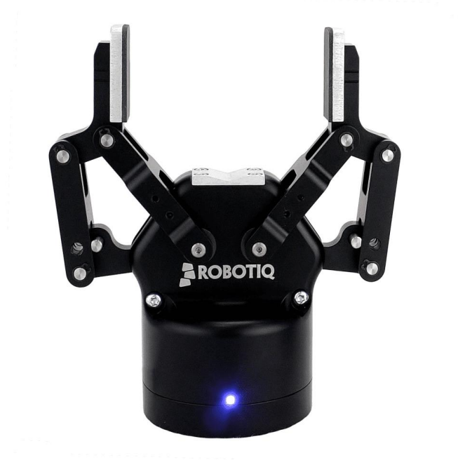
Figura 9: Garra 2F-85 Robotiq
