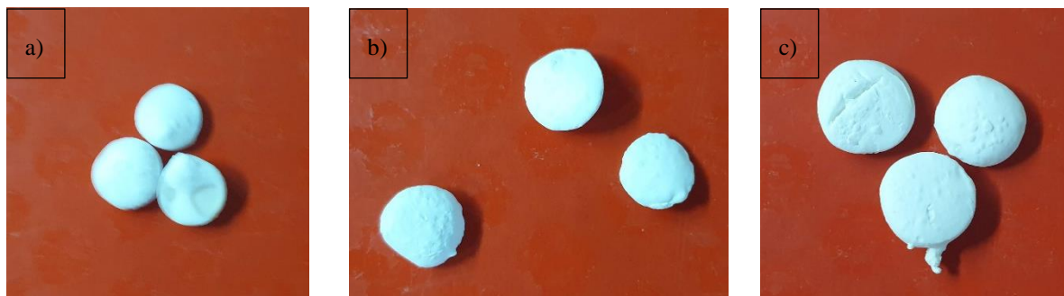
Figure 3.1 Coated aerogels after supercritical drying; a) Pectin b) Alginate c) Alginate and Pectin
