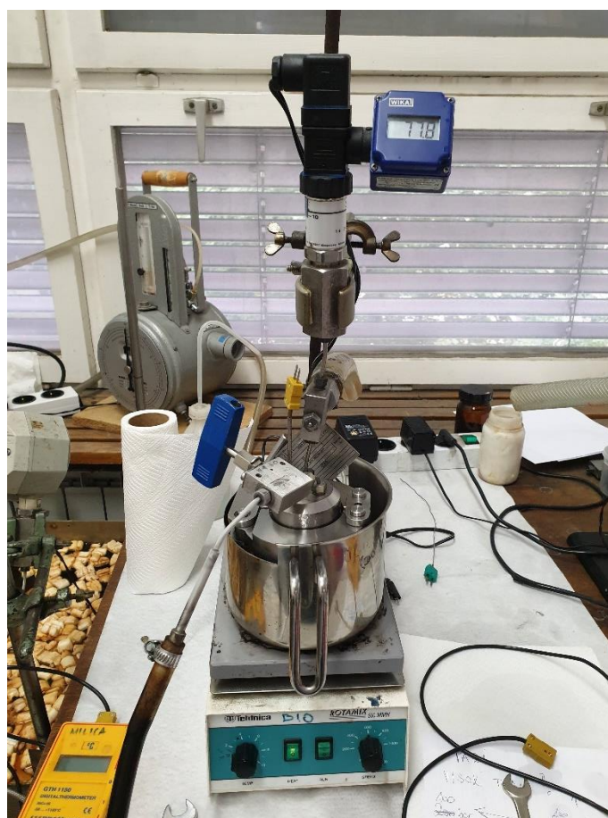
Figure 2.5. Supercritical impregnation apparatus
