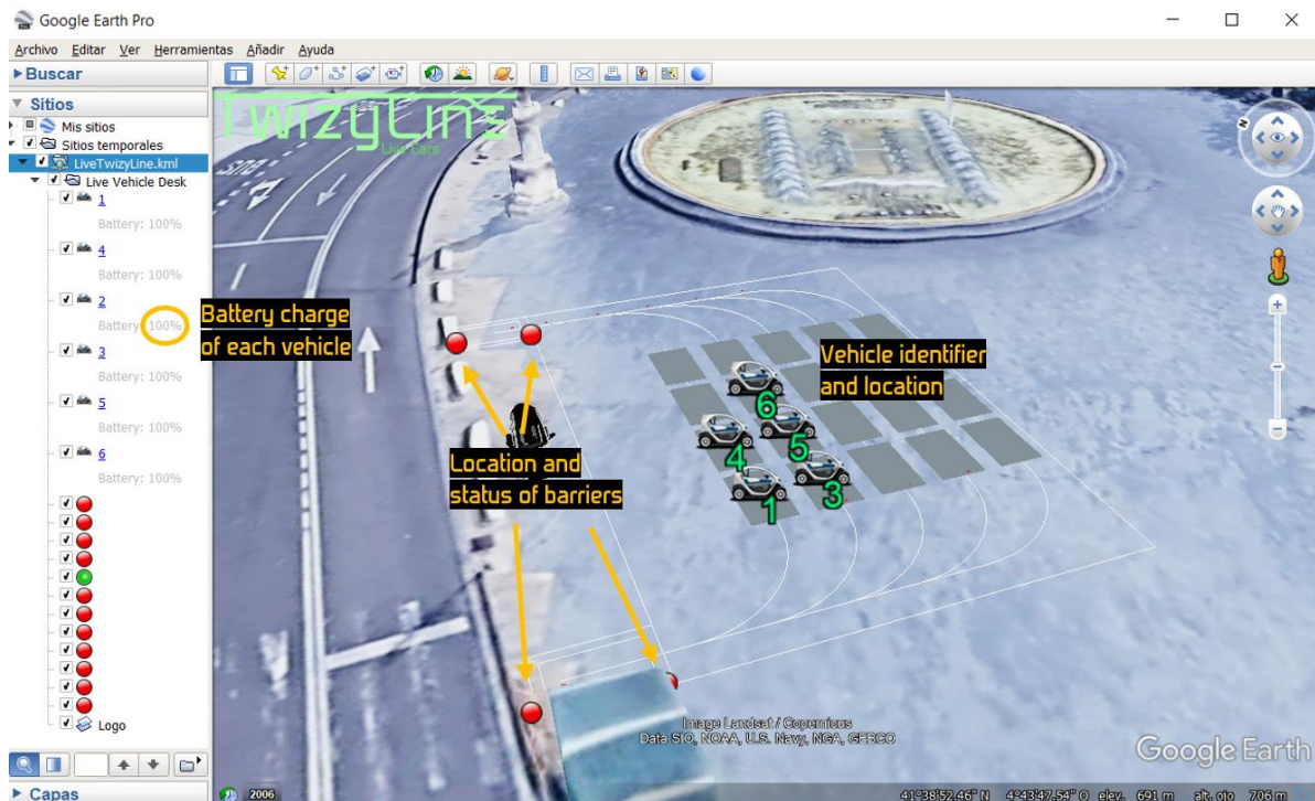
Figure 41. Example of the real-time display of the system status using Google Earth as KML viewer.
