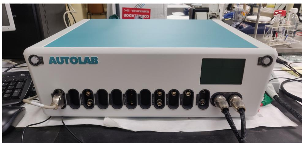
Figura 15: potenciostato PGSTAT 128N (Autolab).
