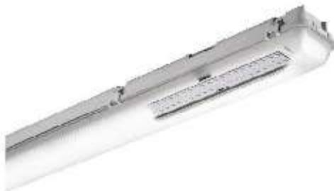
Tufflite LED+ High Efficiency, Surface mounted IP66 luminaire, nominally 1282mm long, 4000K LED with efficiency's up to 156lm/w. Complete with polyester GRP body and polycarbonate opal reeded diffuser
