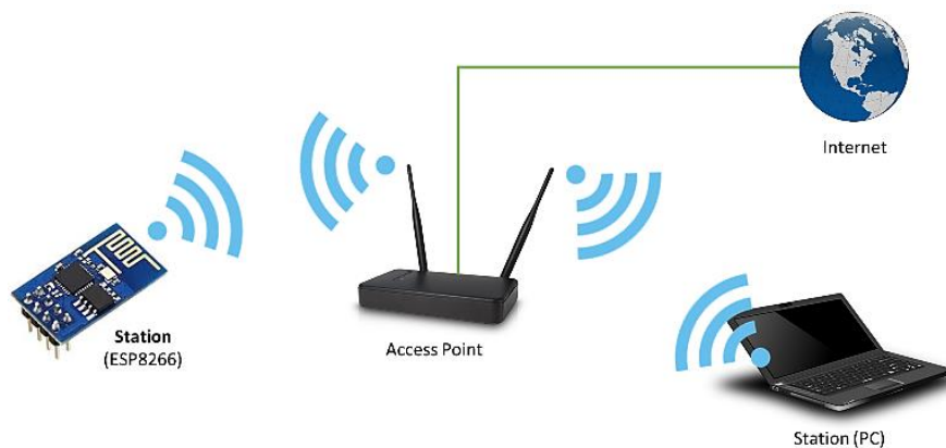
ESP8266 operating in the Station mode
