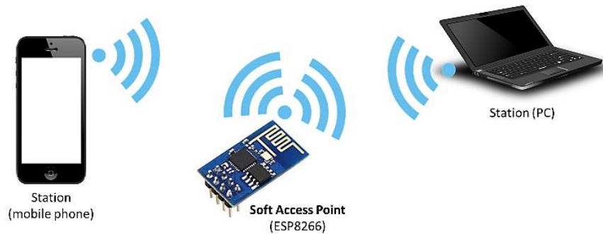
ESP8266 operating in the Soft Access Point mode
