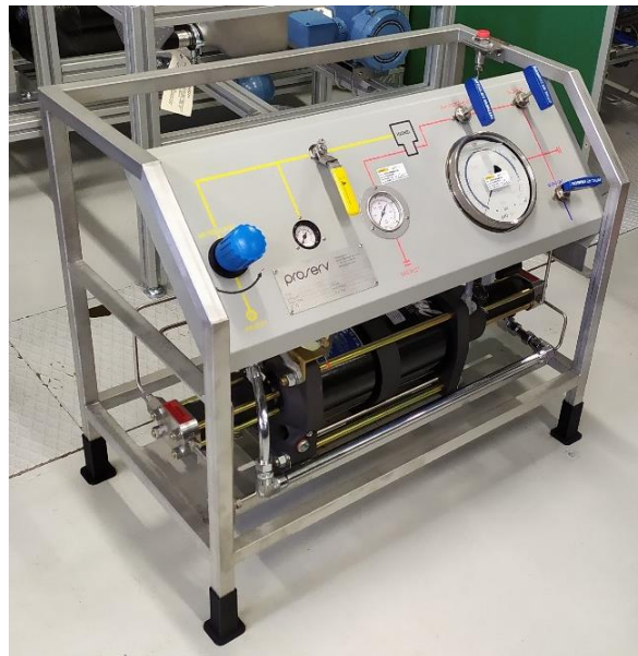
Figure 29 Elevated booster pump
