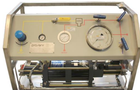
Figure 23 Booster pump HASKEL AGT-62/152H
