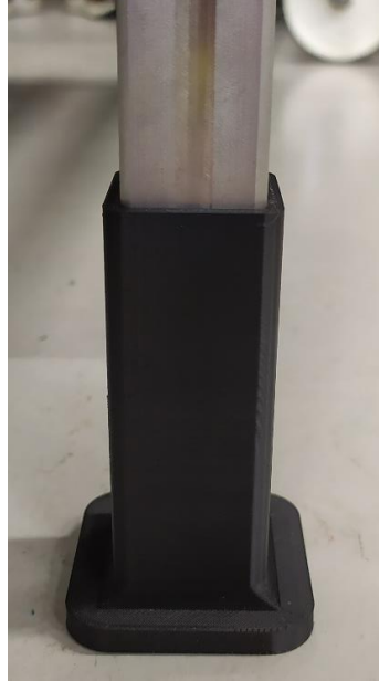
Figure 28 Support fitted in the leg
