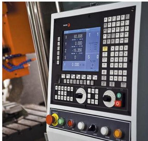
Figura 3.41: Panel de control Fagor CNC 8055. Fuente : Directindustry.
