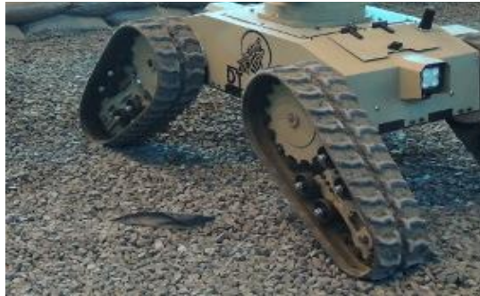
Figure 3.2- 1: Testudo's caterpillar wheels 11
