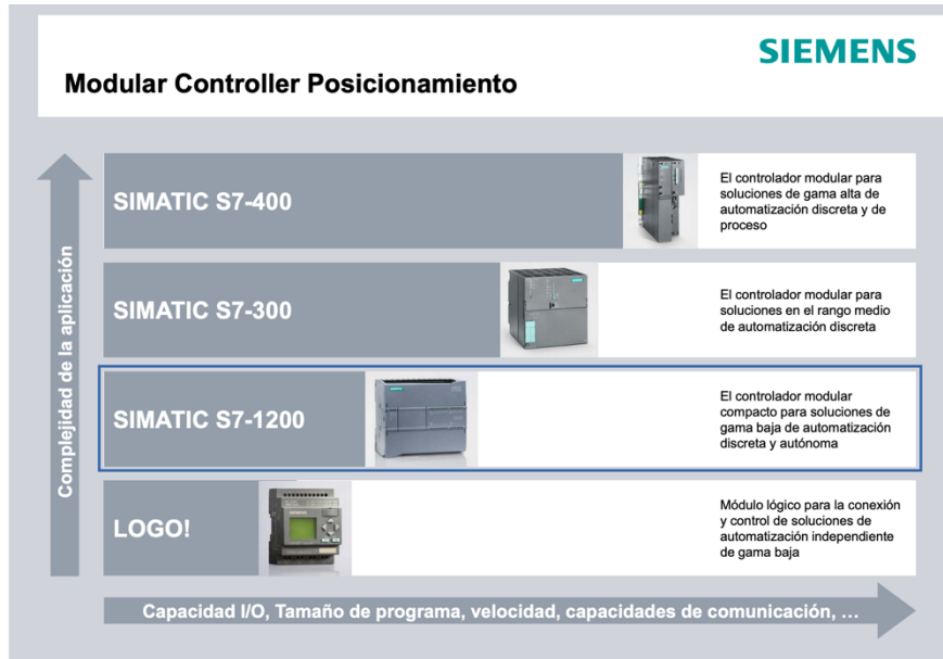
Figura 2.2. Gama PLC SIMATIC S7
