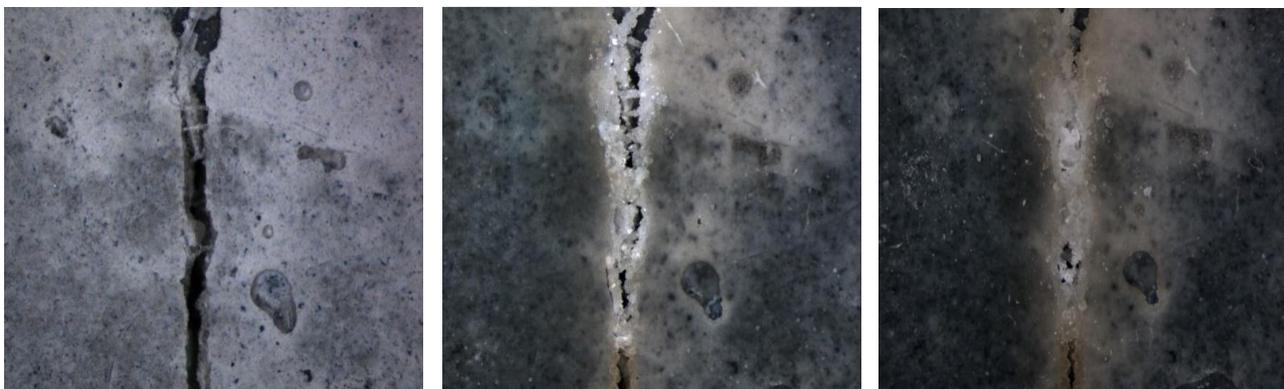
Figura 5. Hormigón autorreparable [Recuperado de CNN – *The ‘living’ concrete that can heal itself*]
