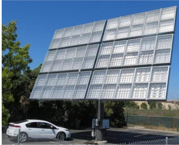
Figure 43: uM6 solar power generator composed by 6 x uM modules [61].
