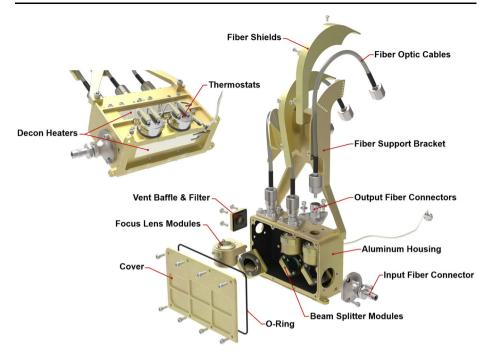
Fig. 7 Rendering of the optical demultiplexer which accepts light from the FOC (at the connector at the right) and distributes it efficiently to the three spectrometers through three fiber bundles
