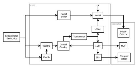
Fig. 28 Simplified schematic diagram of the high-voltage power supply that operates the intensifier depicted in Fig. 14. MCP = micro-channel plate
