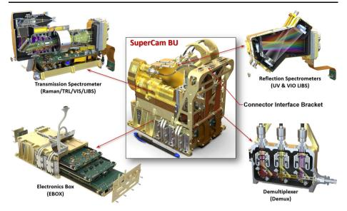
Fig. 4 Subassemblies of the Body Unit
