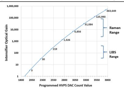
**Fig. 37** Gain produced across the SuperCam intensifier as a function of the digital-to-analog count value (0–4095). The typical DAC setting for LIBS is 2500; Raman spectroscopy uses a DAC setting of 3200, but these can be adjusted, depending on conditions, e.g., decreased to avoid saturation or increased to highlight a weak feature
