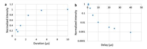
**Fig. 43** Example of the ability of SuperCam to use time resolution to study LIBS processes. Shown are trends in the intensity of the CaF molecular peak measured at 603 nm as a function of the exposure duration up to  $10 \,\mu s$  (**a**), and with up to  $40 \,\mu s$  delay, on a log scale (**b**). In (**a**), all exposures start at a delay of  $800 \, ns$ . In (**b**), all exposures have a duration of  $10 \,\mu s$
