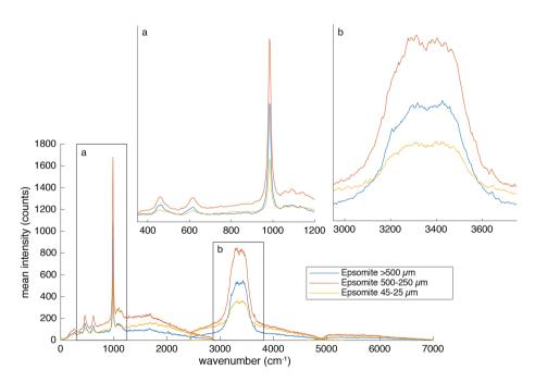
**Fig. 48** SuperCam Raman spectra of pressed-powder pellets of different grain sizes of epsomite, observed with the EQM at 2.25 m distance integrating 100 laser pulses. Wavenumbers are approximate. Insets show closer detail of the fingerprint (a) and water regions (b) of the spectrum
