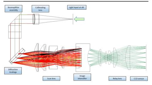
**Fig. 13** Ray traces in a model of the transmission spectrometer, showing collimation, diffraction, and formation of slit images on the image intensifier entrance window and relay lens carrying intensified image to CCD sensor. Rays are colored by wavelength; 534 nm to 853 nm to the intensifier, and 545 nm from the intensifier phosphor to the CCD
