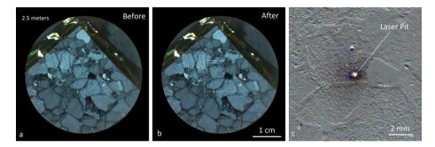
**Fig. 53** RMI images taken during STT of a composite target (62% Ilmenite, 38% Hematite) at 2.6 m, using 19 ms integration time. (a) Before LIBS, 30 shots. (b) After LIBS. (c) Difference of the two images to highlight the laser pit. This level of detail is expected of most RMI images taken in the rover's arm work zone and slightly beyond
