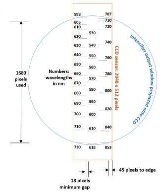
onto the photocathode of the ICCD sub assembly. The images of the slit on the ICCD face are magnified 1.22 times by the scan lens assembly.
