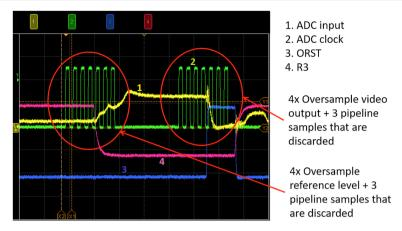
Fig. 26 Oscilloscope traces illustrating the correlated quadruple sampling used to improve the signal-to-noise ratio. ORST is output reset pulse; R3 is readout register phase-3 clock pulse
