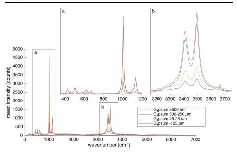
**Fig. 47** SuperCam Raman spectra of pressed-powder pellets of different grain sizes of selenite gypsum (Glitter Mine, Utah), observed with the EQM at 2.25 m distance integrating 100 laser pulses. Wavenumbers are approximate. Insets show closer detail of the fingerprint (**a**) and water regions (**b**) of the spectrum
