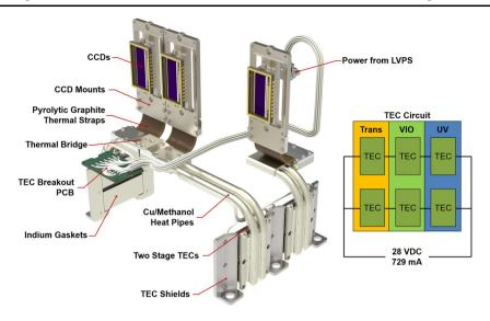
**Fig. 20** The system for cooling the CCDs shown in isolation along with the wiring schematic. The TEC shields provide both protection to the TECs during rover integration and improve the thermal path to the mounting fasteners
