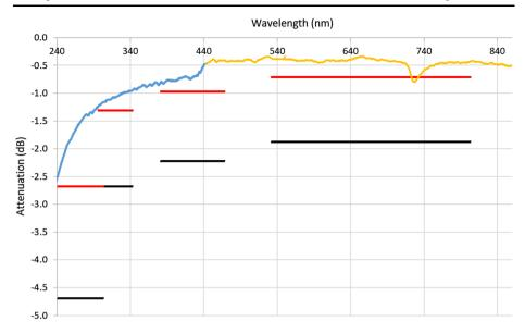
Fig. 6 Attenuation and insertion loss for the flight fiber-optic cable, measured with two commercial spectrometers (orange and blue curves), made after planetary protection/contamination control bake-out and flight-acceptance thermal cycling. Red and black lines indicate goal and requirement levels, respectively
