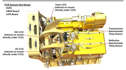
Fig. 22 Locations of all the SOH temperature sensors on the SuperCam BU. Locations were chosen to provide the best temperatures for calibration. Trans = transmission spectrometer
