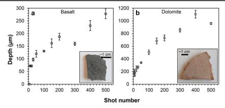
**Fig. 44** Measured pit depths as a function of the number of laser shots for basalt (**a**) and dolomite (**b**) made with the EQM laser at a distance of 2.86 m in a simulated Mars atmosphere. Error bars show the standard deviations of three pits at each number of shots. Insets show the samples. Rows of pits can be seen in the dolomite sample (**b**)
