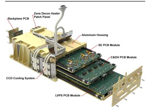
**Fig. 18** An exploded view showing the major components of the electronics box (EBOX). Its back-plane/daughter-card architecture allows easier removal and installation of circuit boards during assembly and testing. The EBOX acts as the support structure for the optical sub-assemblies
