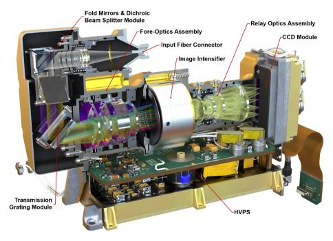
Fig. 14 Cutaway rendering of the transmission spectrometer showing the internal layout
