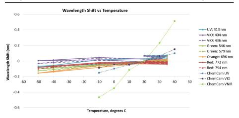
Fig. 39 Shift of the position of the incident light on the CCDs as a function of temperature. Construction with titanium instead of beryllium (ChemCam) resulted in a large improvement in thermal stability
