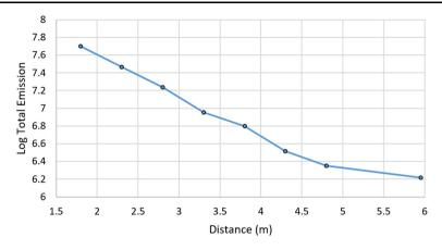
Fig. 42 Total emission from target JA-1 as a function of distance
