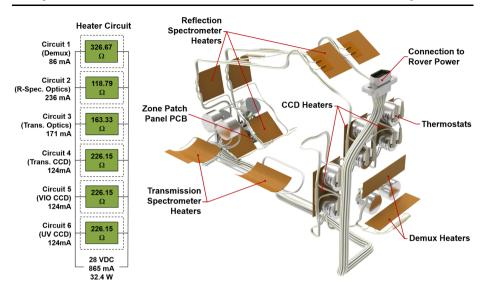
Fig. 21 Decontamination heater system shown in isolation along with the wiring schematic. The system is composed of six independent zones, each controlled by a pair of redundant thermostats and operating on rover power
