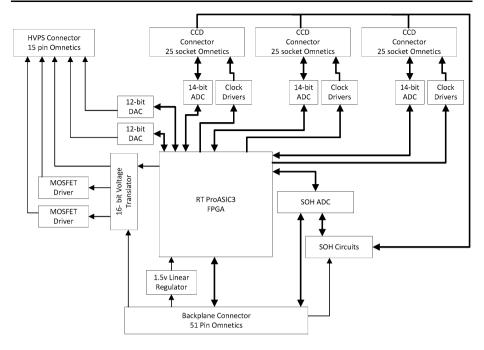
**Fig. 25** Schematic diagram for the BU spectrometer electronics board. ADC = analog-to-digital converter; DAC = digital-to-analog converter; Op Amp = operational amplifier; MOSFET = metal-oxide semiconductor, field-effect transistor. See main text for the meaning of other abbreviations
