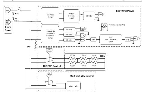
Fig. 23 Schematic diagram of the BU low-voltage power supply. RTN = return; EMI = electromagnetic interference; Cap = capacitor; LC = inductance-capacitance
