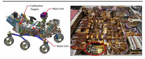
Fig. 3 Locations of the SuperCam units on the rover. The right side shows the rover body inverted, with the Body Unit circled. It is next to the RSM side of the rover to minimize the length of the fiber that transfers the optical signal from the mast unit. The rover's instrument and electronics bay is  $1181 \times 1106$  mm (length, left-right, x width)
