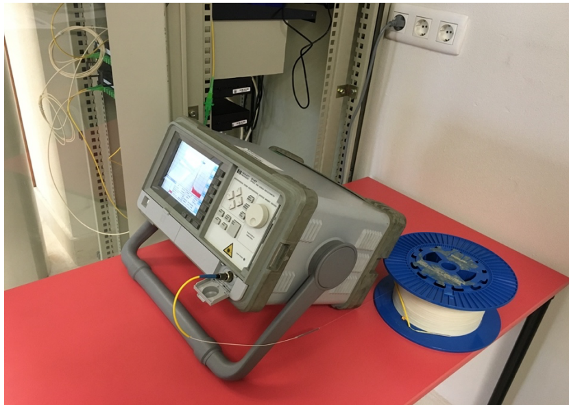
Figure 21. Appearance of the launch fiber just after the OTDR.
