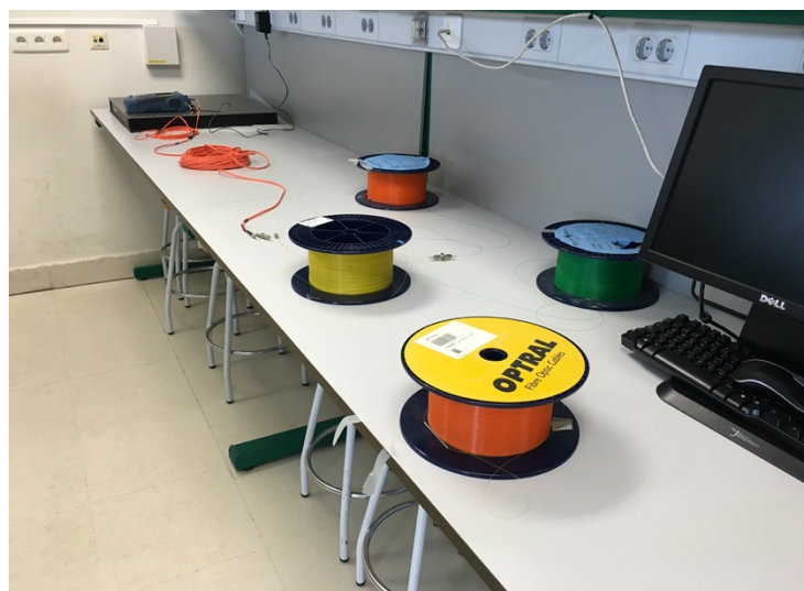
Figure 15. Multimode fiber link to be characterize using the OTDR
