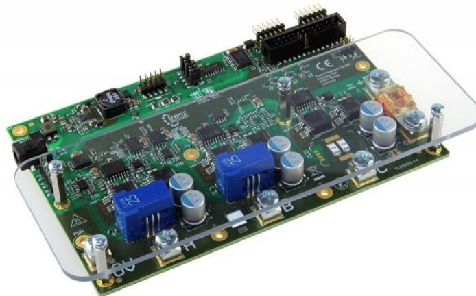
Figura 120. Inversor EDPS Power Stage
