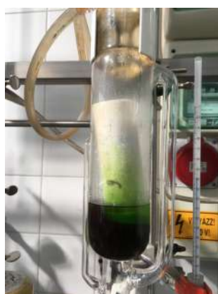
Figure 22. Soxhlet extraction in progress with thyme and 96%EtOH.
