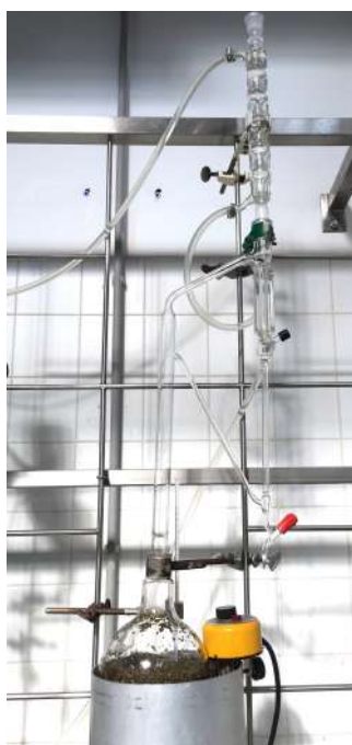
Figure 19. Hydrodistillation. Clevenger apparatus in the laboratory.
