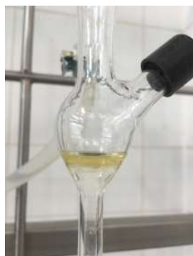
Figure 18. Distilled essential oil in the Clevenger apparatus.
