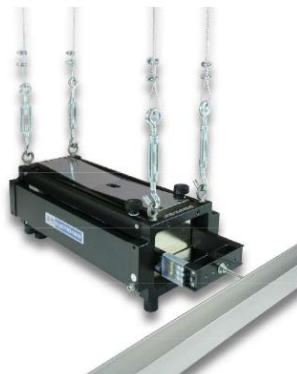
APS 113 with APS 8610 - Modal Stinger and APS 8611 - Steel Cable Kit prepared for Free Body Mode operation
