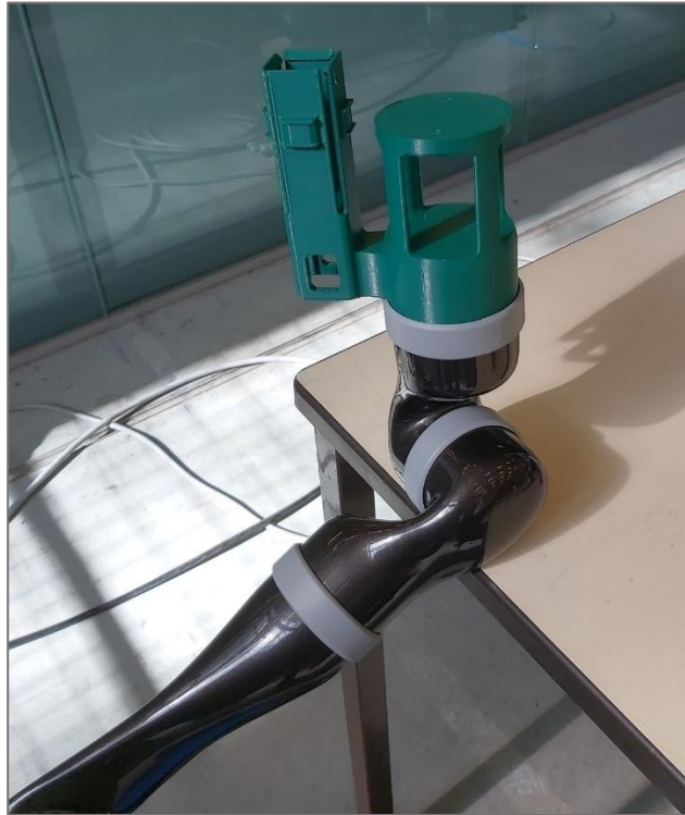
Figure 4.4. 3D printed model included in the robot arm located on the ARCHER robot.
