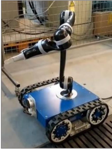
Figure 2.9. Execution of joint position control on the ARCHER robot arm.
