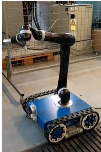
Figure 2.13. Execution of service command on the ARCHER robot arm.
