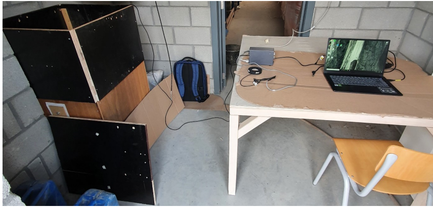
FIGURE 3.18: Nijst equipment setup for database creation, including opaque box, lighting, camera, power supply and computer.
