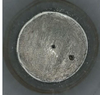
Figure 49 Bottom covered with paint
