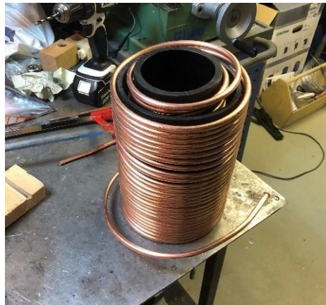
Figure 39 Bending process TES 2
