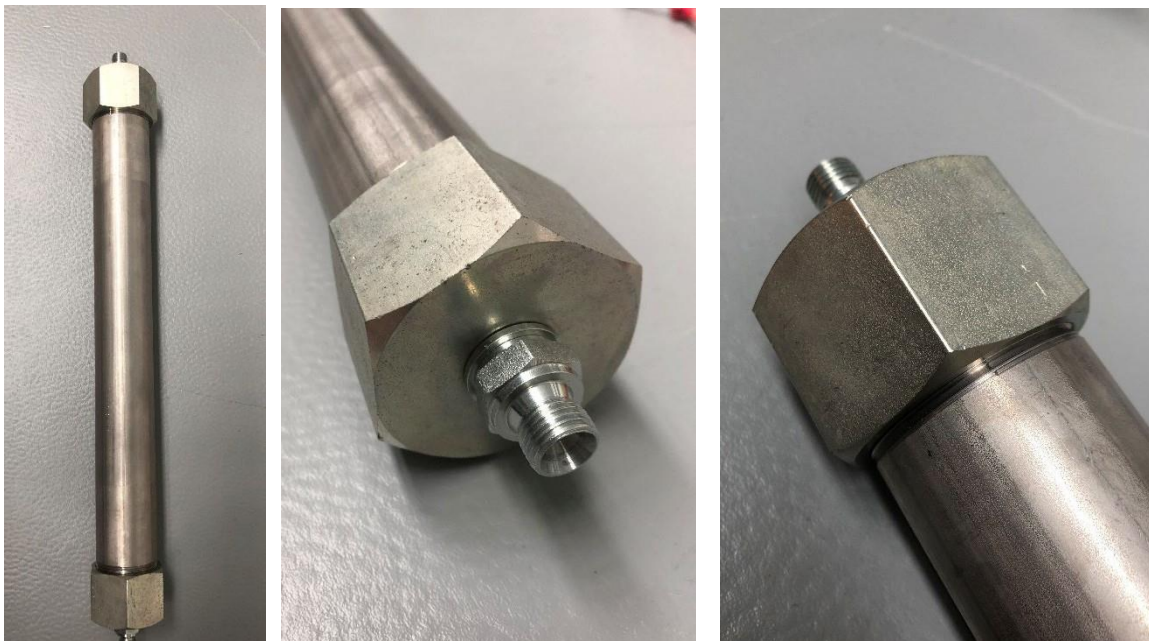
Figure 67 Final result of the air vessel and the connectors
