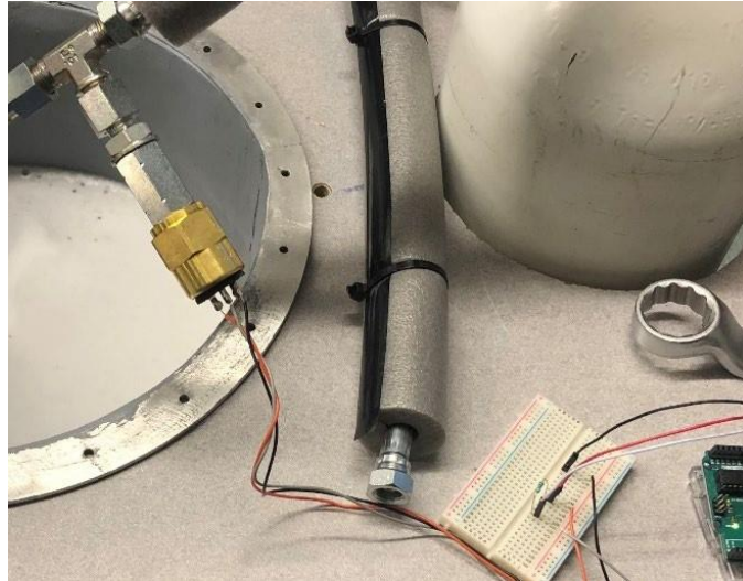
Figure 59 Pressure sensor on demo
