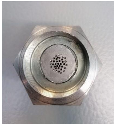
Figure 68 Drilled holes in filter
