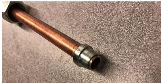
Figure 41 Cutting Ring Fitting
