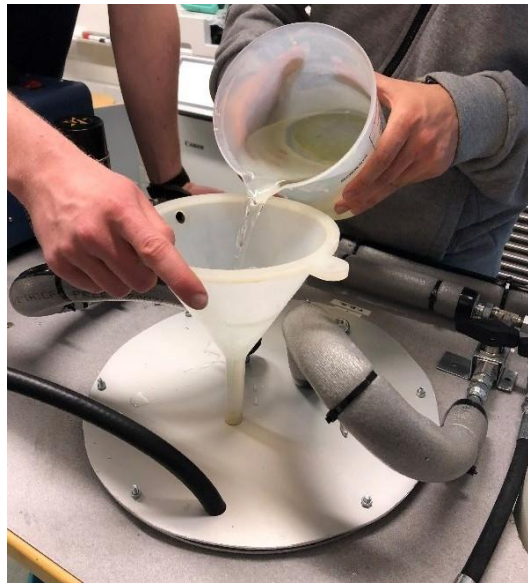
Figure 76 TES tank filled up with water
