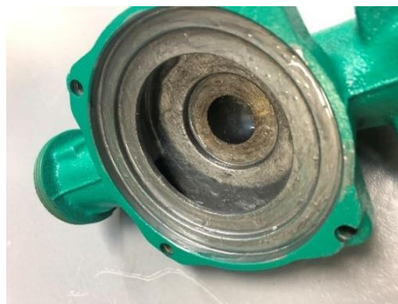
Figure 35 Inside of pump painted
