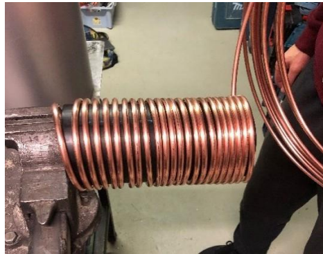
Figure 38 Bending process TES 1
