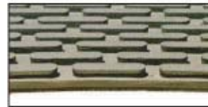
Raised lozenges pattern (for rough calibration)
