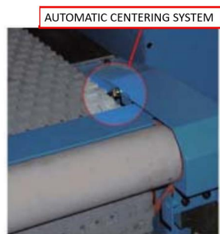
Figure 11.4. Automatic centring system of the wood sheets in the Series K calibrating sanding machine by Costa Levigatrici.
