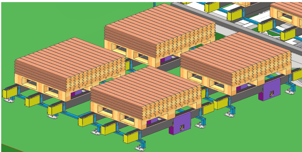
Figure 7.31. Image of the two existing conveyors at the beginning of the line.
