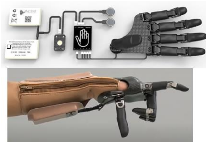
Figura 11. Componentes y brazaletes del Vincent Partial Hand. [16]
