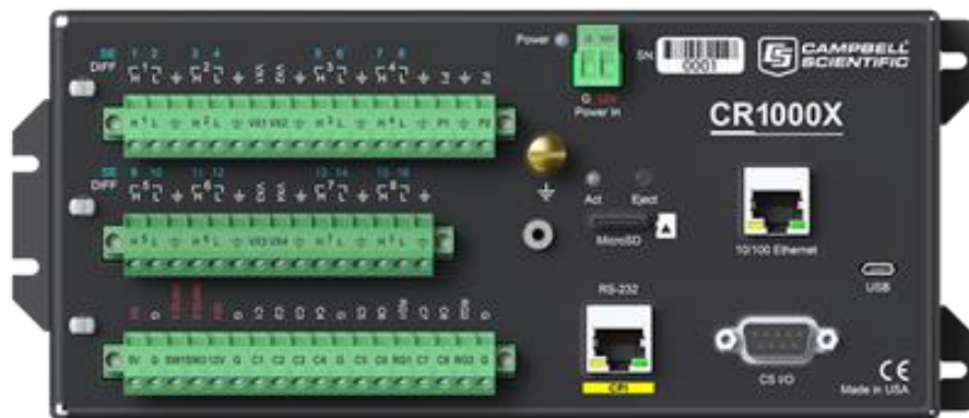
Figure 37. Campbell Scientific CR1000 data logger [37]
