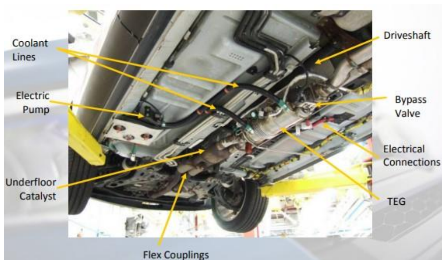
Figure 34. Illustration of the car with its different parts [33]
