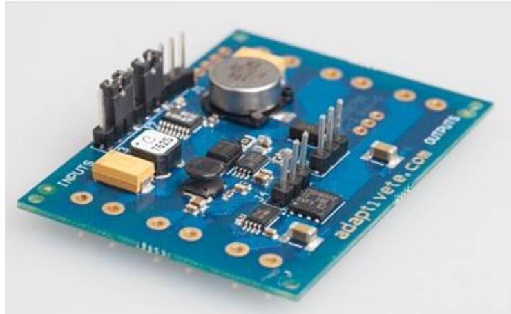
Figure 45. Energy Harvesting Board ADEH-P-A [38]
