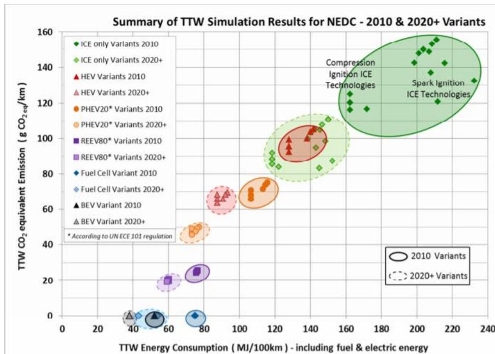
Figure 15: TTW Emissions and Energy Consumption in 2010 and 2020 by vehicle type
