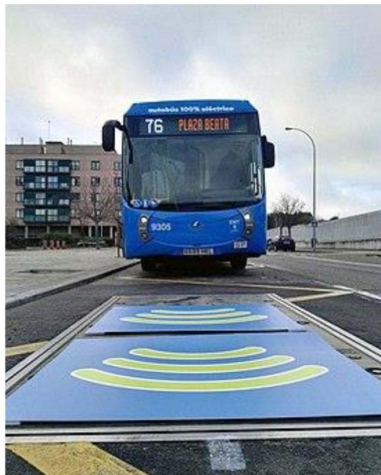
Figure 13: Wireless charging system and E-bus in Madrid (ETRA, s.f.)
