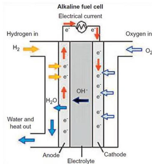
Figure 8: Functioning of a fuel cell (Breeze, 2017)
