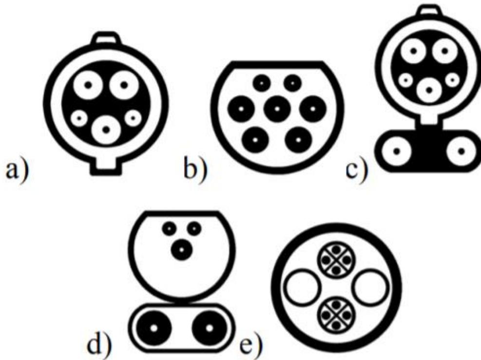
Figure 12: Standardized connectors for EVs (Raff et al. 2019)
