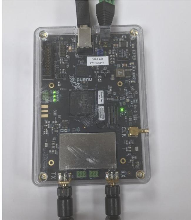
Figura 4: FPGA *BladeRFx40*
