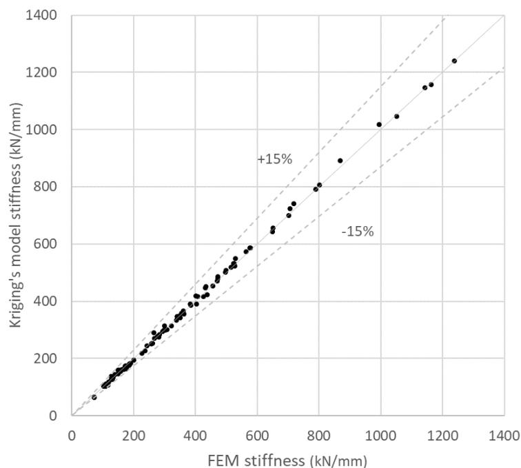
**Figure 2.** Stiffness comparison between FEM and Kriging's model.
