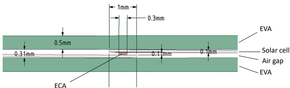
**Figure 1.** Cross-sectional view of connection region of two solar cells
