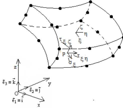
**Figure 1.** Finite Element of 20 nodes. The Cartesian coordinates system and the representation of the isoparametric system  $\{\zeta \ \eta \ \xi\}$ .
