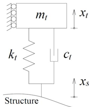
Figure 1. Schema of a SDOF system attached to a certain point of a structure.
