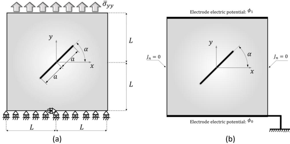
**Figure 1.** (a) Cracked plate of MWCNT/epoxy composite material subjected to uniform tension. (b) Position of the electrodes on the plate.
