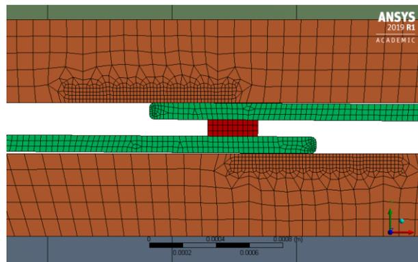
**Figure 2.** Finite Element model of solar cells (green), ECA (red) and EVA (brown)
