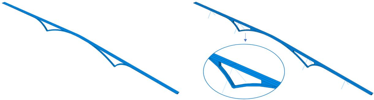
**Figure 2.** FE ABAQUS model before (left) and after reinforcement (right)
