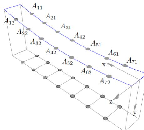
**Figure 1.** Footbridge model. Location of the accelerometers.
