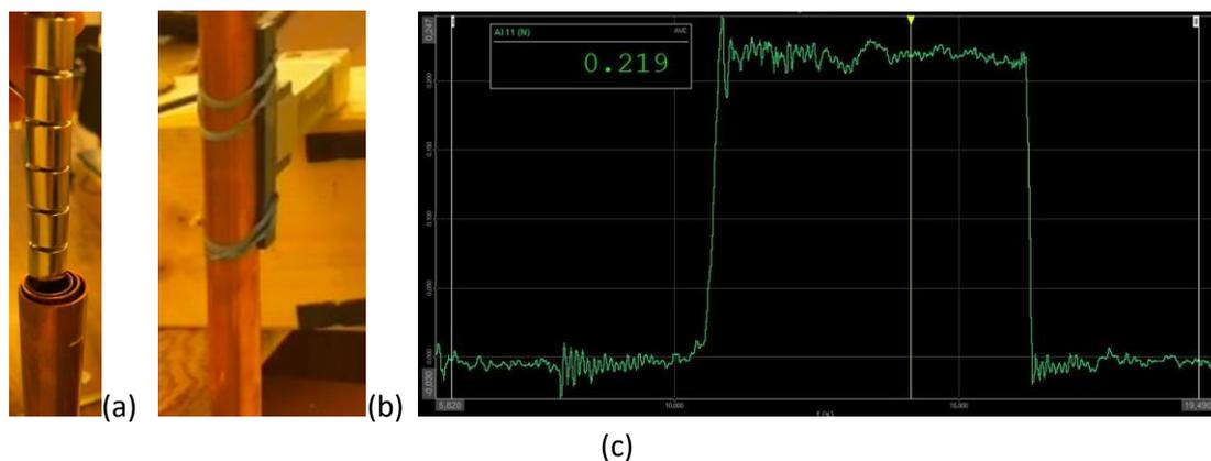
**Figure 2.** Experimental layout. Pile of magnets (a) load cell (b) and force vs. time records (c)
