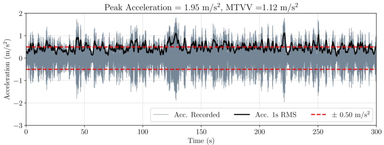
**Figure 2.** Response of FRP footbridge at midspan due to three pedestrians walking freely.
