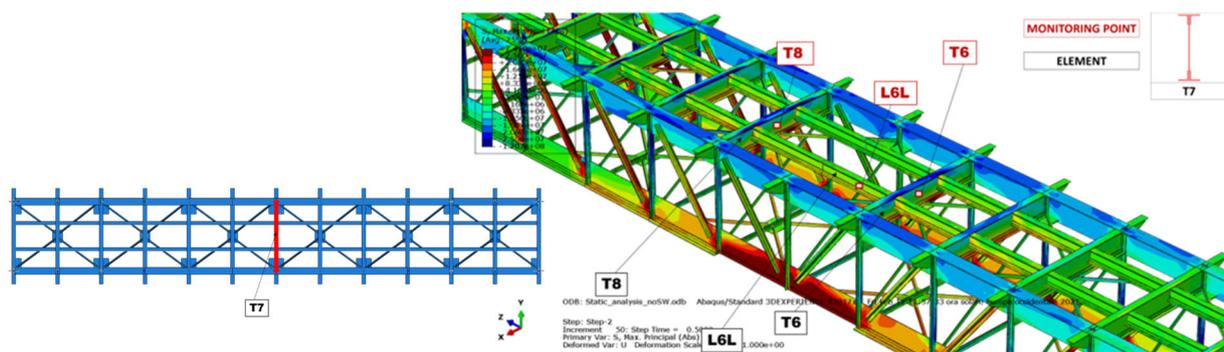
**Figure 2.** Preliminary results obtained with the LSA analysis carried out on Abaqus.
