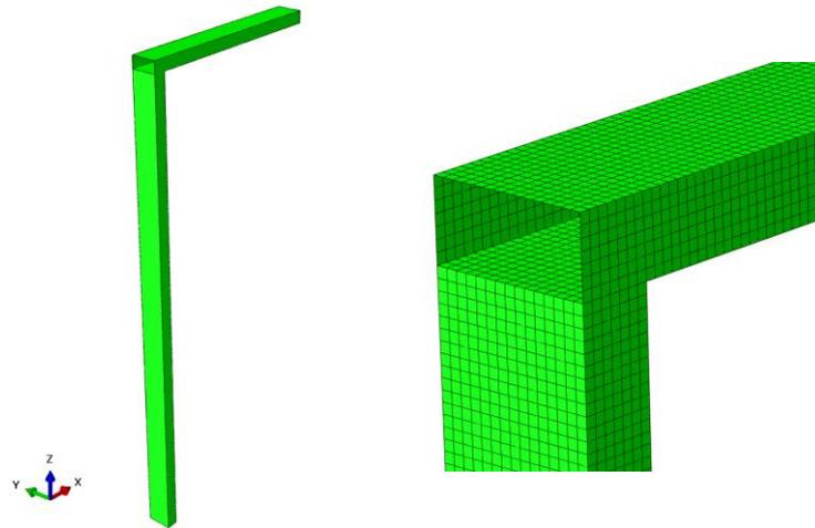
**Figure 2.** Numerical shell model (ABAQUS)
