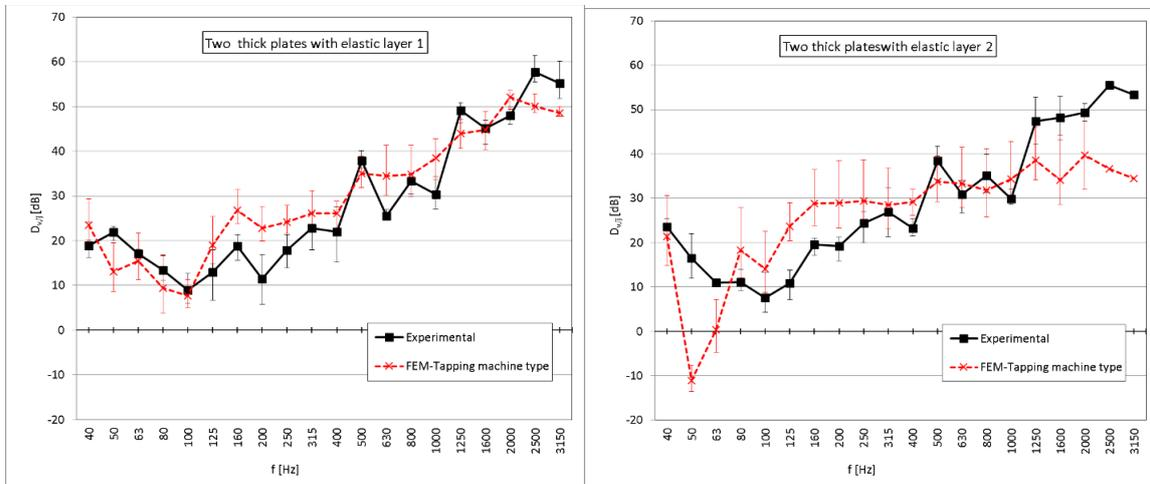
**Figure 2.** Velocity level difference: two thick plates. Elastic layer 1 and 2. Average of three excitations and maximum and minimum values.
