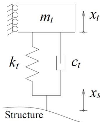
Figure 1. Schema of an ideal TMD modelled as an SDOF system
