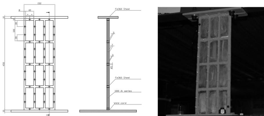
**Figure 2.** Prototype of the aluminium-steel dissipater.
