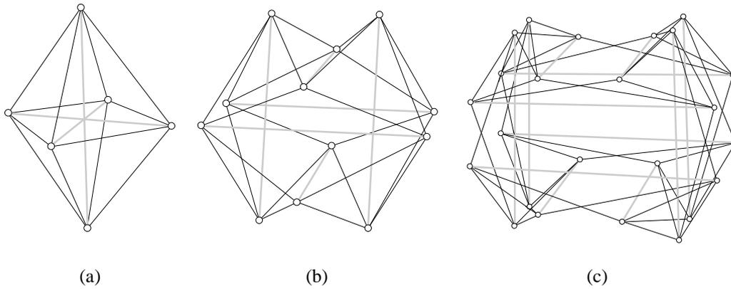
**Figure 1.** Octahedron family: (a) octahedron, (b) expanded octahedron and (c) double-expanded octahedron. Black lines correspond to cables and grey lines to struts. Adapted from [7].
