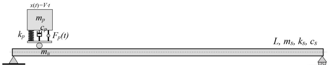
Figure 1. Mass-Spring-Damper system for Human-Structure interaction model.
