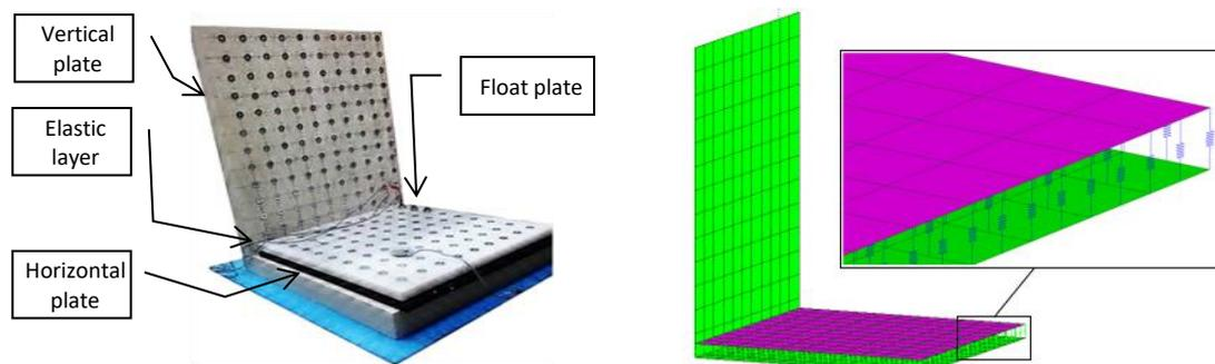
**Figure 1.** Geometry of the joint connecting thick plates and floating plate and models with elastic layer (mesh for the plates and for the elastic layer).
