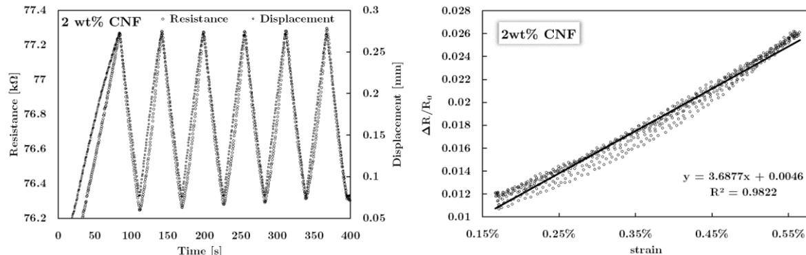
**Figure 2.** Resistance variation during static cycling tensile load (left). Unit resistance variation vs. strain (right).
