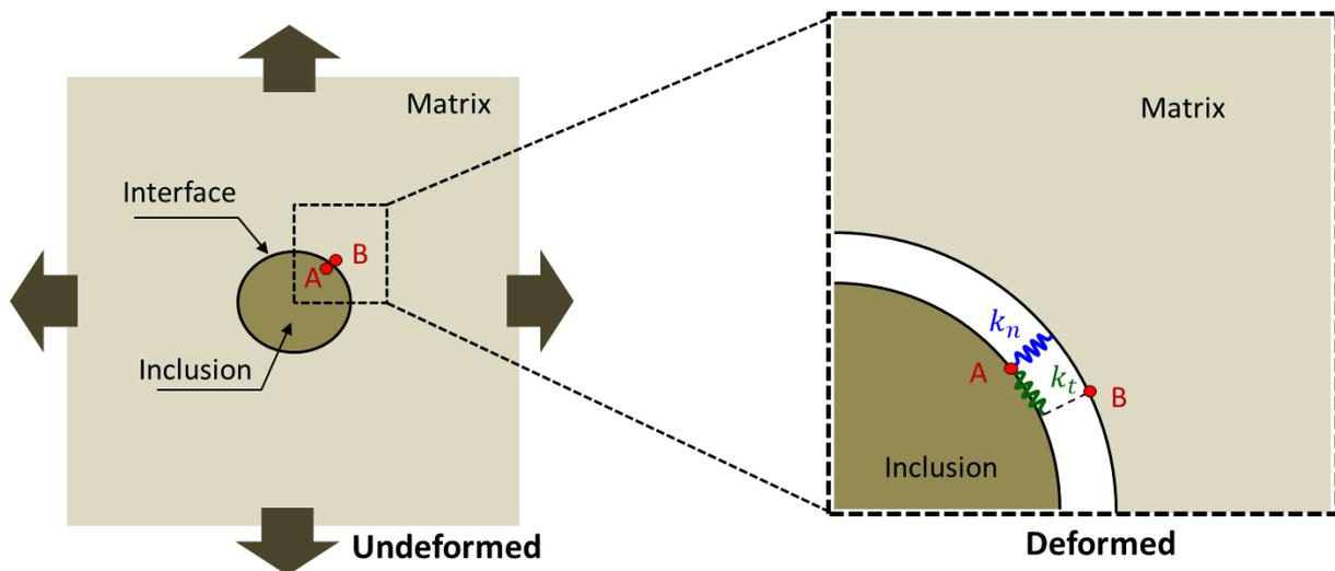
Figure 1. Scheme of the matrix-inclusion interface spring model proposed in [3, 4].
