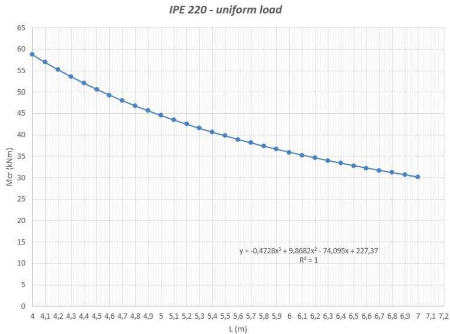
**Figure 1.**  $M_{cr}$ -L curve for IPE 220, with  $L = 4\text{-}7\text{m}$ , under uniform load.
