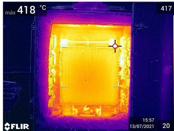
*Figure 1. Masonry panels submitted to high temperature.*
