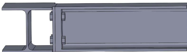
**Figure 1.** *Beam-to-beam connection with additional plate.*
