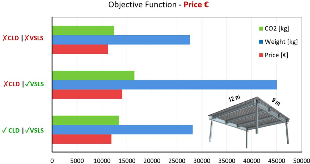
**Figure 2.** Structural Optimization Results for a 12m X 9m composite floor with and without checking the VSLS and with and without considering the CLD viscoelastic treatment studied.
