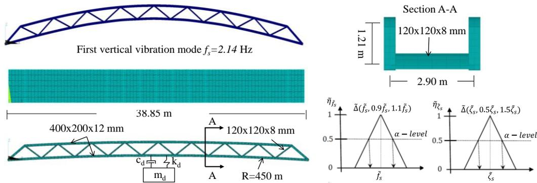
**Figure 1.** Description of the benchmark footbridge, first vertical vibration mode and triangular membership functions,  $\tilde{\Delta}$ , of the two fuzzy variables (where  $\tilde{f}_s$  is the first vertical natural frequency and  $\tilde{\zeta}_s$  is the associated damping ratio) considered to simulate the uncertain conditions.
