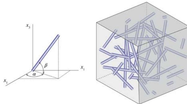
**Figure 1.** RVE of a short fiber-reinforced composite material, with  $\alpha$  and  $\beta$  being the Euler angles used to represent the relative orientation of the fillers.
