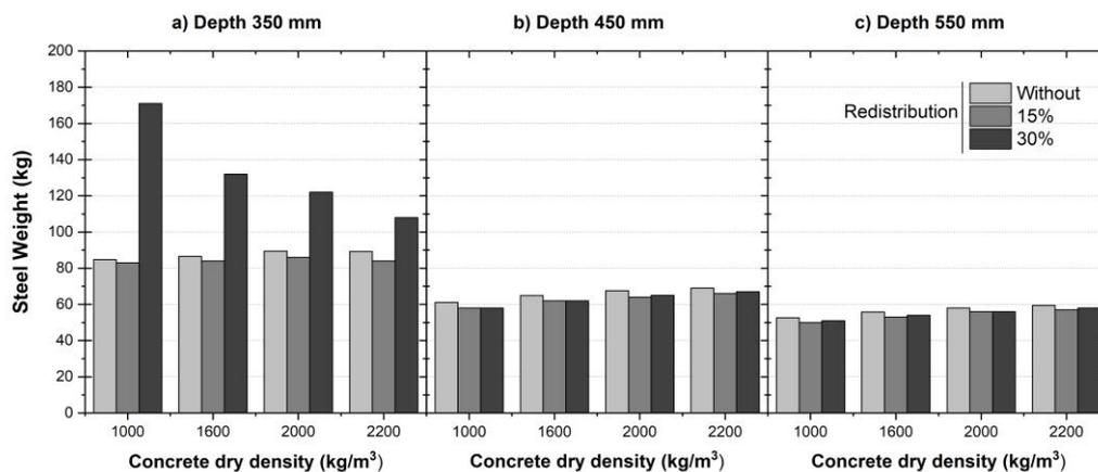
Fig. 1 Effect of concrete density and moment redistribution factor on the longitudinal reinforcement savings for a 5 m two-span continuous beam with  $f_{ck} = 25$  MPa and subjected to an occupancy load of 2 kN/m<sup>2</sup>.
