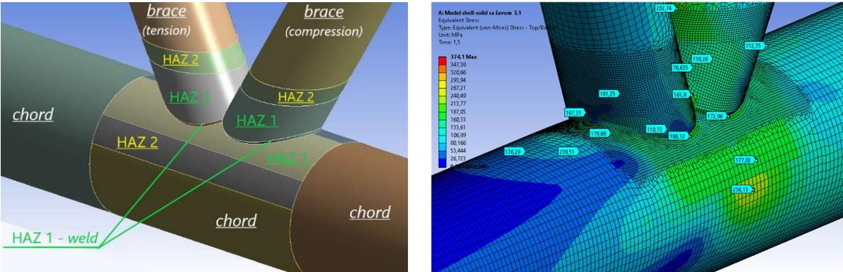
Figure 3. a/ Position of aluminium softening zones HAZ 1 and HAZ 2. b/ An example of Von Mises equivalent stress in the most loaded K-joint
