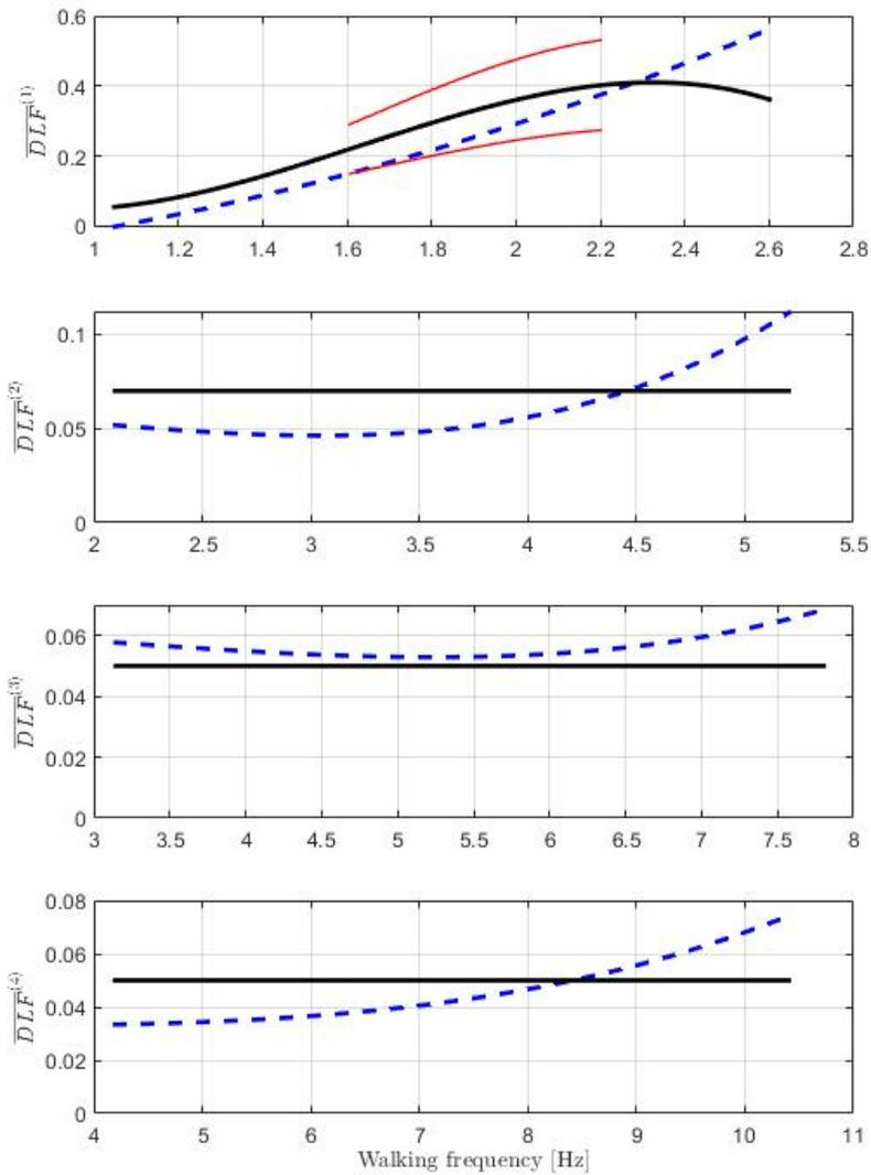
**Figure 1.** Determinist component of DLF vs walking frequency. Solid lines: Kerr's study. Bold line: averages, Fine line: 95% confidence bounds. Dashed lines: present study..
