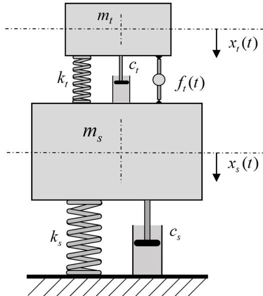
Figure 1: Dynamic system of model of a TMD with a force device.
