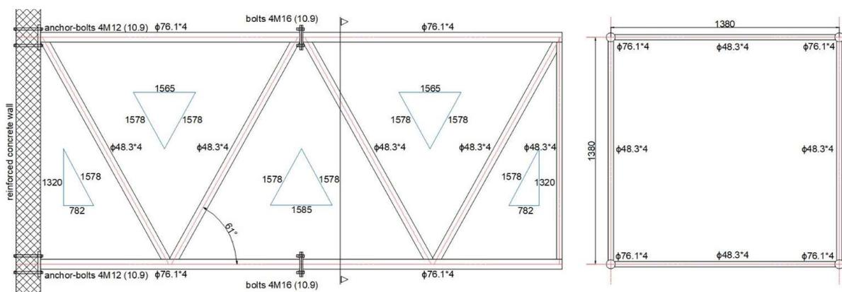
**Figure 1.** General geometry of analysed spatial aluminium lattice structure made of CHS profiles with uniplanar K-joints.
