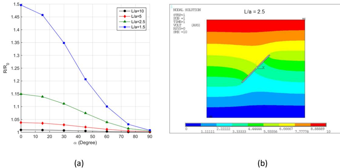
**Figure 2.** (a) Influence of crack size ( $L/a$ ) and crack orientation ( $\alpha$ ) on changes in electrical resistance. (b) Distribution of the electric potential in the plate for the case of a crack size of  $L/a = 2.5$  and a crack orientation  $\alpha = 45^\circ$ .
