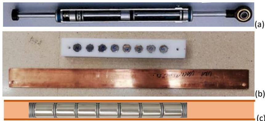
**Figure 1.** Different types of dampers. (a) viscous damper. (b) axial magnetic device. (c) radial piston-like magnetic damper.
