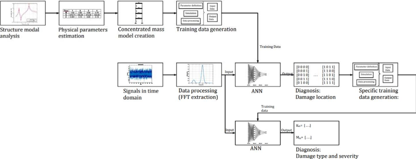
Figure 1: Scheme of the proposed methodology
