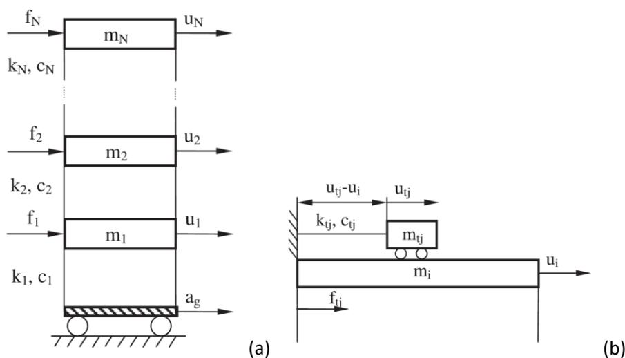
Figure 1. Conceptual N-storey building (a) and TMD models (b)
