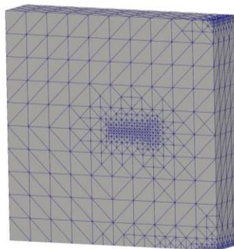
**Figure 1.** Example of the refined mesh
