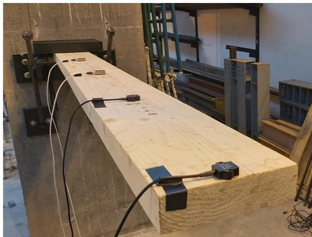
**Figure 2.** *Dynamic analysis of a structural element of wood.*
