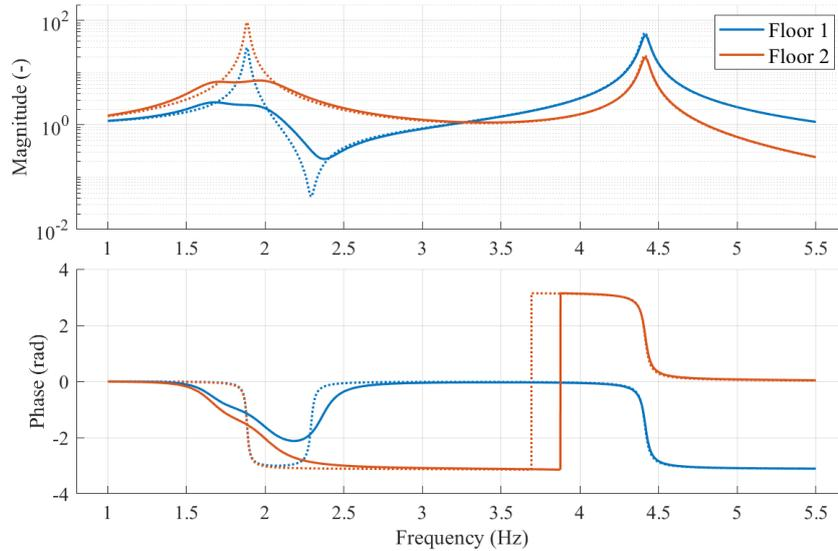
**Figure 1.** FRF in terms of acceleration for the original building (dotted) and for the building with a TMD (solid).
