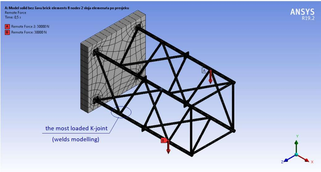
Figure 2. ANSYS model of analysed spatial lattice structure.
