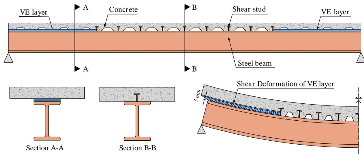
Figure 1. Studied CLD treatment applied to composite floors.
