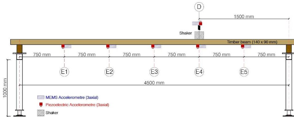
**Figure 1.** Validation test for a simple version of the system
