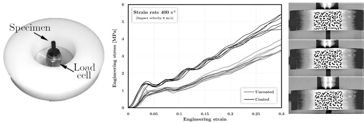
**Figure 1.** Rubber pellets ready for impact test (left); during impact test (right). Test results for coated and uncoated pellets (center)
