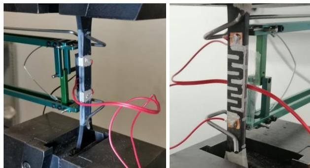
**Figure 1.** Specimens of enriched resin under tensile test.
