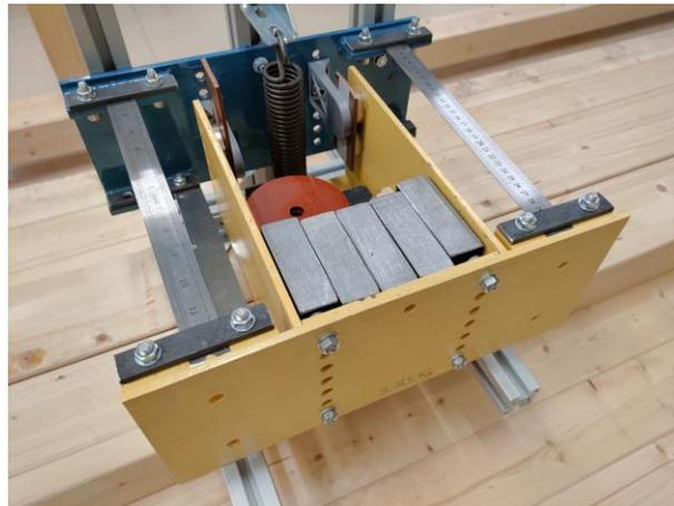
**Figure 2.** Experimental realization of the TMD used to validate the methodology.
