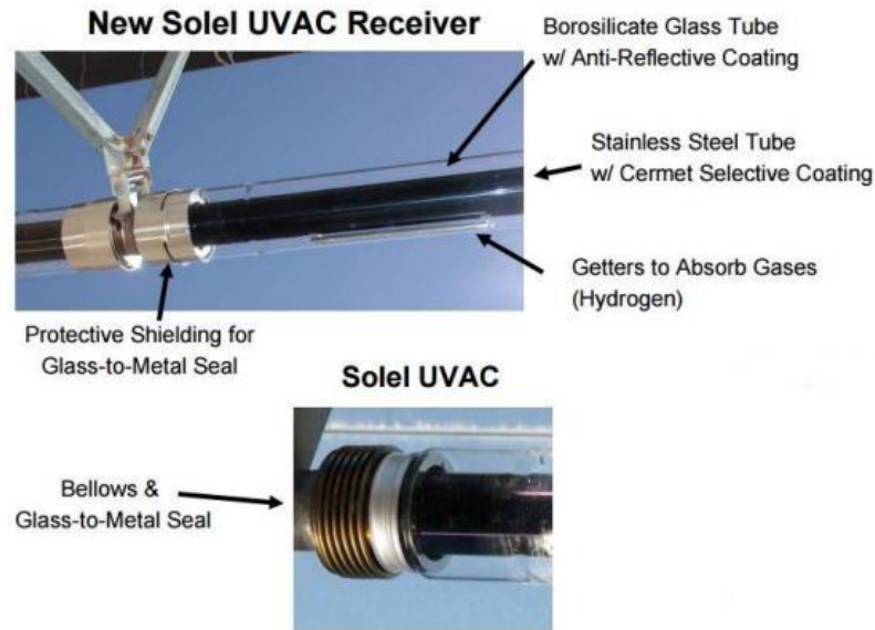
Figura 39. Receptor Solel UVAC [54]
