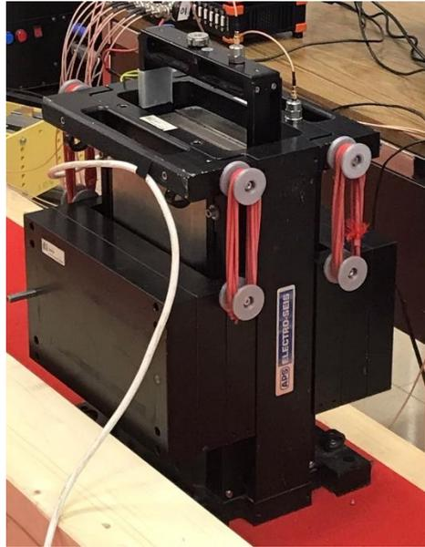
*Figura 3.5. Shaker APS 400 ELECTRO-SEIS.*
