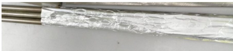
Figure 5.10 metal structure of 3 bars closed with aluminium to support FTO.
