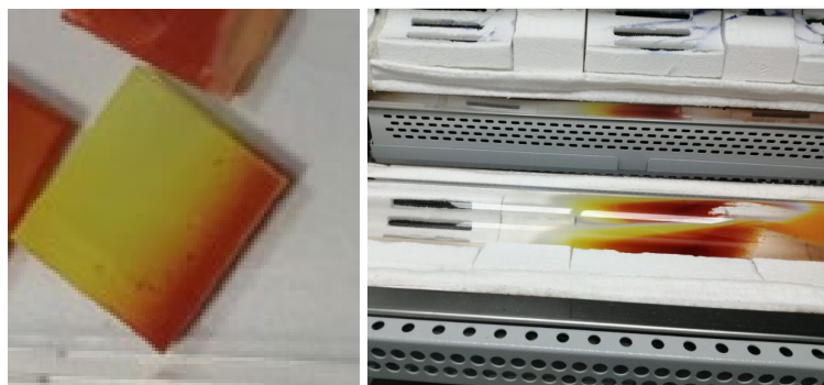
Figure 5.3 image of the yellow compound generated at 400 °C and image of the tube after the experiment
