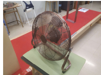
d) Fan used as structure exciter
