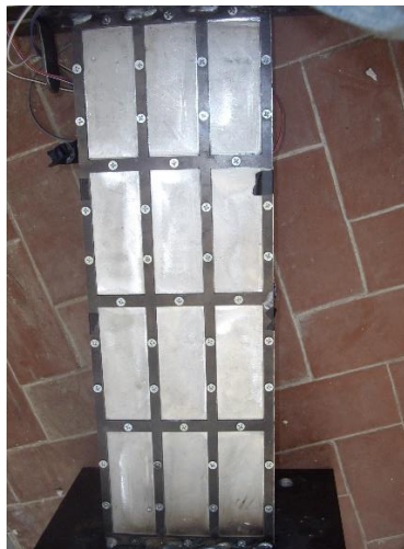
Figure 2. Aluminum - steel dissipator with 12 windows ( N_c = 3 , N_r = 4 ) and w_1 = 8\text{mm} , w_2 = 40\text{mm} , w_3 = 8\text{mm} , h_1 = 10\text{mm} , h_2 = 100\text{mm} , h_3 = 10\text{mm} , s_1 = 5\text{mm} , s_2 = 3\text{mm} , s_3 = 2\text{mm} .
