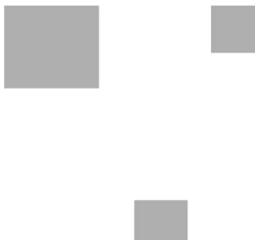
Figure 2.14: Configuration space of a point-sized robot. White = C_{free} , gray = C_{obs} (from Simeon87 (2008))
