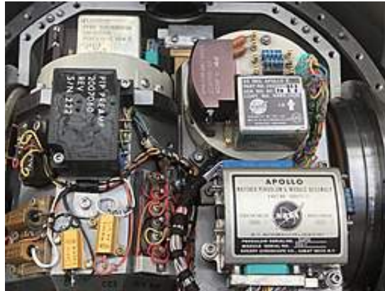
Figure 2.7: Apollo IMU stable member (Reinhold (2019))
