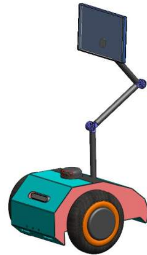
Figure 3.7: ATEMR: Mobile Base Design - 3D design v1 ISOMETRIC VIEW
