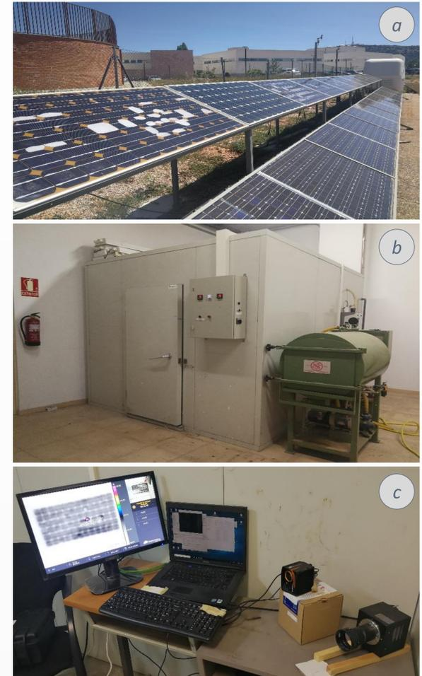
Figure 1: PV field of the Campus Duques de Soria (a), temperature and humidity controlled chamber at the EIFAB in Soria (b) and EL and IR imaging capturing system used in the temperature and humidity controlled chamber ©
