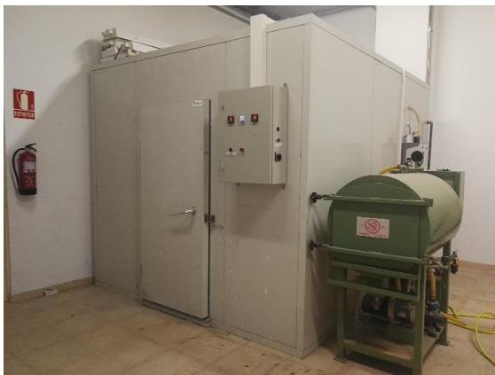
Figure 1: Temperature and humidity controlled chamber at the EIFAB in Soria, Spain
