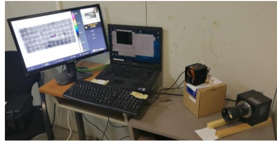
Figure 2: EL and IR imaging capturing system used in the temperature and humidity controlled chamber
