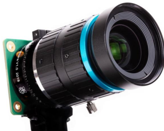
Figure 29. Raspberry Pi HQ Camera with telephoto lens mounted on it
