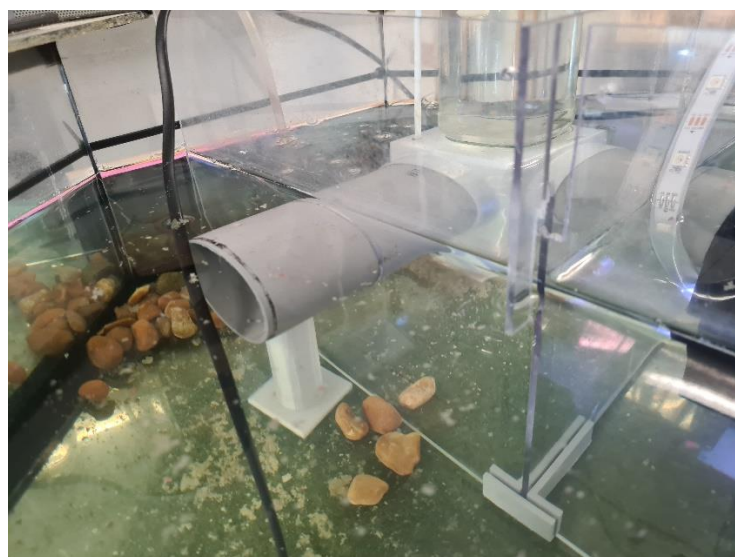
Figure 27. Vision of the support under the pipe and the holding of the plexiglass
