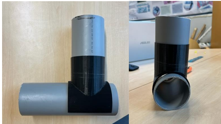
Figure 9. Improvement of the junction with the 3D printed part
