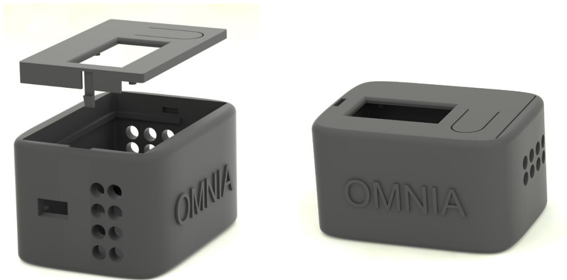
Figure 53 -Renders of the vibration sensor prototype
