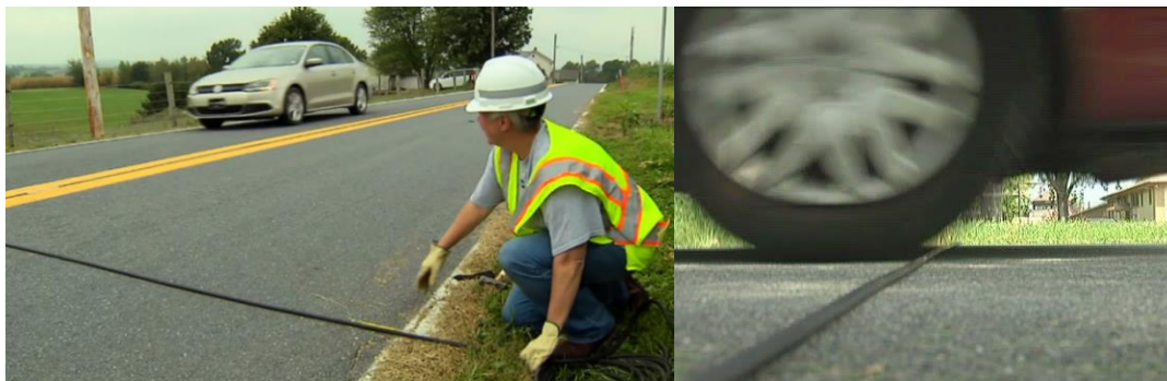
Figure 18- Image of pneumatic tube sensor working
