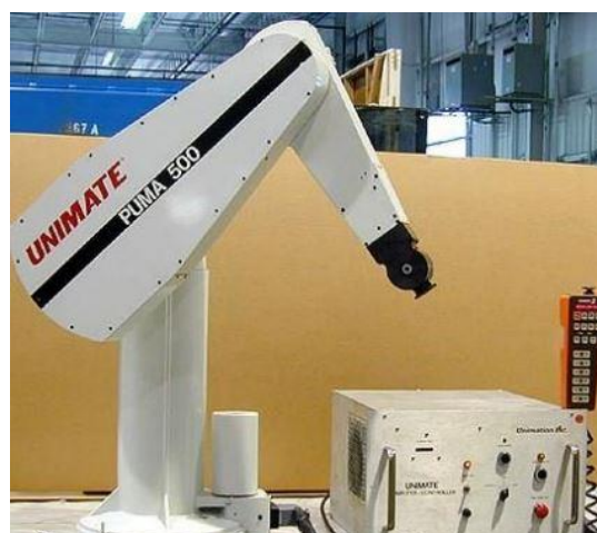
Figura 6: robot PUMA 500 de 6 GDL [21]
