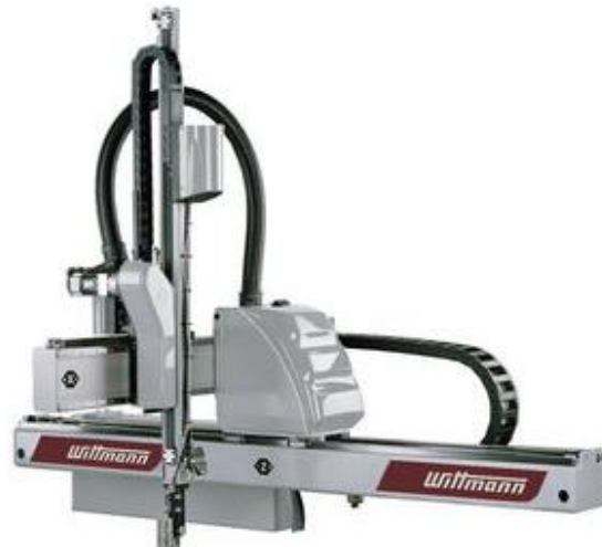
Figura 7: robot cartesiano de 3 GDL [20]
